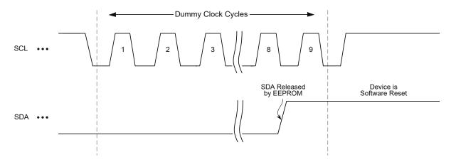
In the event that the device is still non-responsive or remains active on the SDA bus, a power cycle must be used to reset the device (see 4.5.1 Power-Up Requirements and Reset Behavior).
