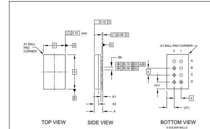
COMMON DIMENSIONS (Unit of Measure = mm)
