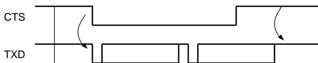
Figure 21-28. Transmitter Behavior when Operating with Hardware Handshaking
