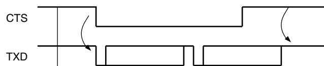
Figure 19-17. Transmitter Behavior when Operating with Hardware Handshaking
