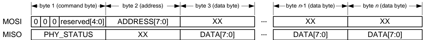
Figure 6-11. Packet Structure – SRAM Read Access.
