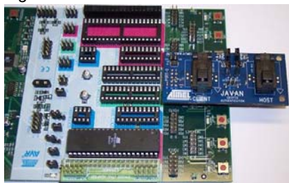
Figure 18. AT88CK109BK3 Mounted to the STK500
