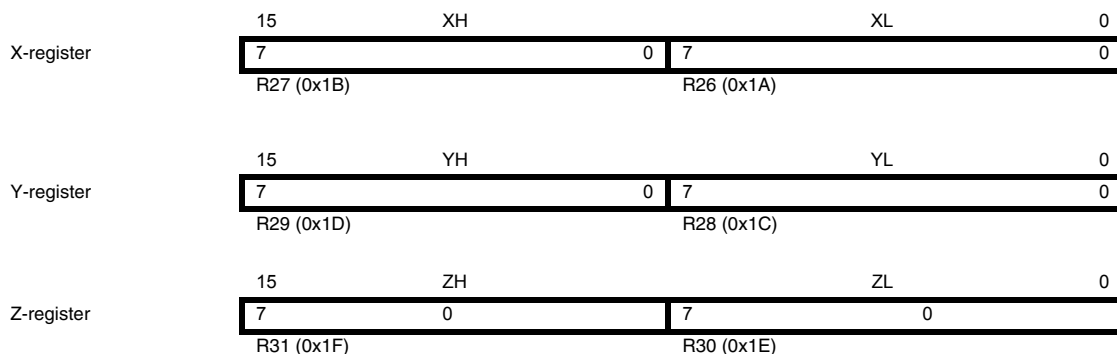
Figure 5-3. The X-, Y-, and Z-registers.
