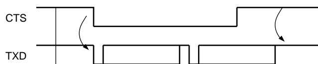
Figure 31-21. Transmitter Behavior when Operating with Hardware Handshaking
