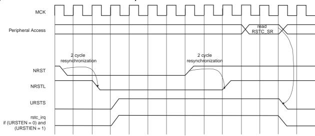
Figure 13-9. Reset Controller Status and Interrupt
