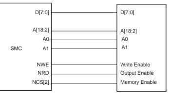
Figure 20-4. Memory Connection for a 16-bit Data Bus
