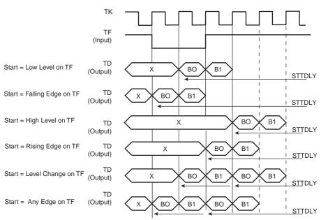
Figure 32-11. Receive Pulse/Edge Start Modes
