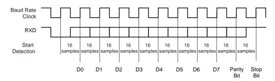
Example: 8-bit, Parity Enabled
