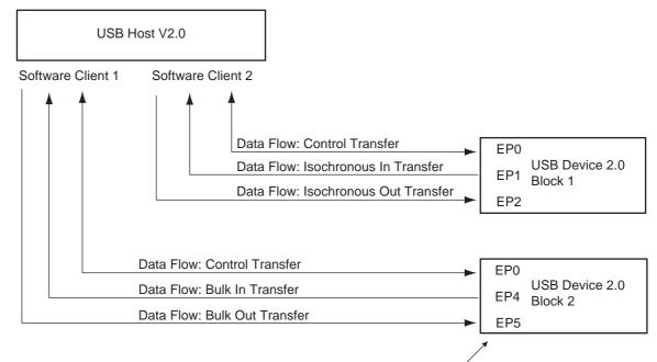
USB Device endpoint configuration requires that in the first instance Control Transfer must be EP0.
