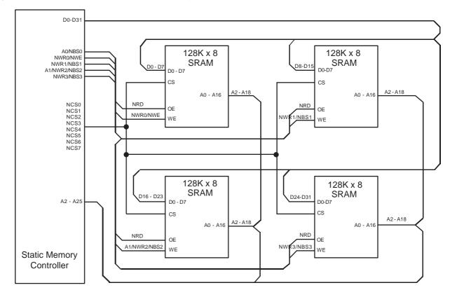
Figure 20-1. SMC Connections to Static Memory Devices
