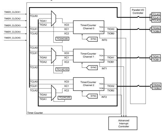
Figure 33-1. Timer Counter Block Diagram
