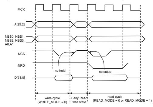
Figure 20-19. Early Read Wait State: NWE-controlled Write with No Hold Followed by a Read with one Setup Cycle
