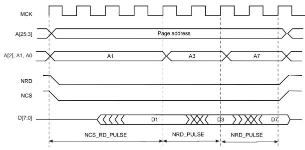
Figure 20-35. Access to Non-sequential Data within the Same Page
