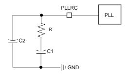
Values of R, C1 and C2 to be connected to the PLLRC pin must be calculated as a function of the PLL input frequency, the PLL output frequency and the phase margin. A trade-off has to be found between output signal overshoot and startup time.
