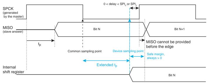
Figure 38-8. SPI Master mode with (CPOL = 0 and NCPHA = 1) or (CPOL = 1 and NCPHA = 0)
