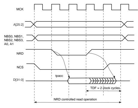
Figure 20-20. TDF Period in NRD Controlled Read Access (TDF = 2)
