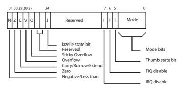
Figure 10-2 shows the status register format, where:
