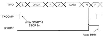
Figure 30-10. Master Read with Multiple Data Bytes
