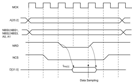
Figure 20-10. READ\_MODE = 1: Data is sampled by SMC before the rising edge of NRD
