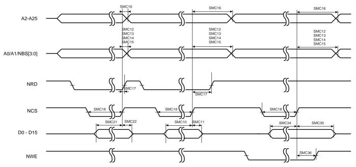
Figure 38-5. SMC Signals for NRD and NWR Controlled Access
