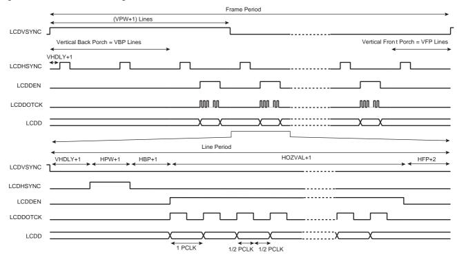
Figure 37-4. TFT Panel Timing, CLKMOD = 0, VPW = 2, VBP = 2, VFP = 1
