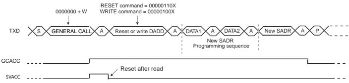
Note: This method allows the user to create an own programming sequence by choosing the programming bytes and the number of them. The programming sequence has to be provided to the master.
