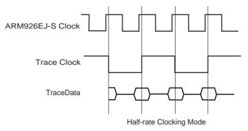
Care must be taken on the choice of the trace capture system as it needs to support half-rate clock functionality.
