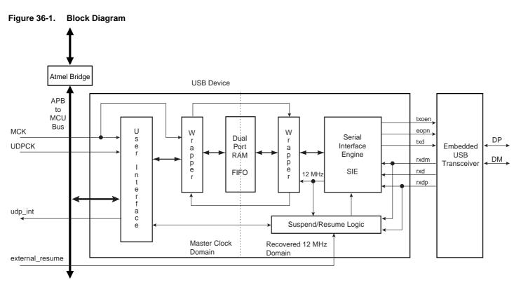
Access to the UDP is via the APB bus interface. Read and write to the data FIFO are done by reading and writing 8-bit values to APB registers.
