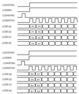
Figure 37-8. Single Scan Monochrome and Color 8-bit Panel Timing (First Line Expanded View)
