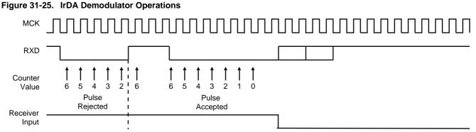
As the IrDA mode uses the same logic as the ISO7816, note that the FI\_DI\_RATIO field in US\_FIDI must be set to
