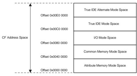
Note: The A22 pin of the EBI is used to drive the REG signal of the CompactFlash Device (except in True IDE mode).
