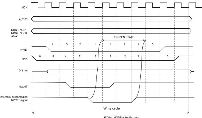
Figure 20-26. Write Access with NWAIT Assertion in Frozen Mode (EXNW\_MODE = 10)
