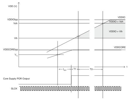
VDDCORE and VDDBU are controlled by internal POR (Power-On-Reset) to guarantee that these power sources reach their target values prior to the release of POR.
