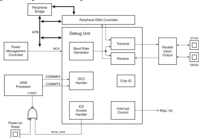
Figure 27-1. Debug Unit Functional Block Diagram
