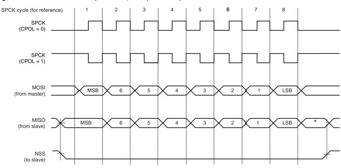
Figure 29-3. SPI Transfer Format (NCPHA = 1, 8 bits per transfer)
