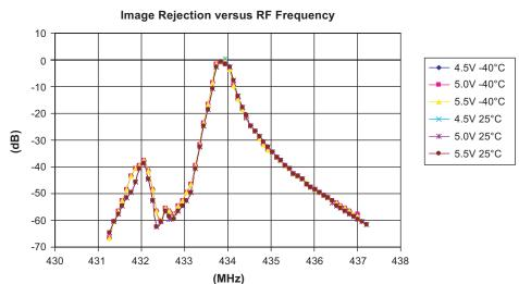
Figure 5-1. Narrow Band Receiving Frequency Response ATA8204
