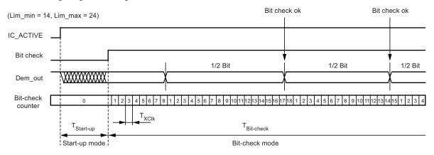
Figure 8-5. Timing Diagram for Failed Bit Check (Condition: CV\_Lim < Lim\_min)
