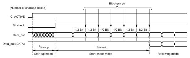
According to Figure 8-3, the time window for the bit check is defined by two separate time limits. If the edge-to-edge time  $t_{ee}$  is in between the lower bit-check limit  $T_{Lim\_min}$  and the upper bit-check limit  $T_{Lim\_max}$ , the check continues. If  $t_{ee}$  is smaller than  $T_{Lim\_min}$  or  $t_{ee}$  exceeds  $T_{Lim\_max}$ , the bit check is terminated and the receiver switches to sleep mode.
