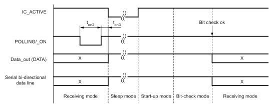
Figure 8-12. Activating the Receiving Mode using Pin POLLING/\_ON
