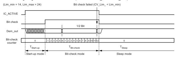
Figure 8-6. Timing Diagram for Failed Bit Check (Condition: CV\_Lim ≥ Lim\_max)
