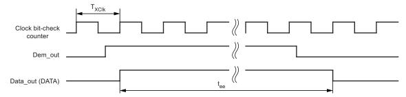
Figure 8-8. Debouncing of the Demodulator Output
