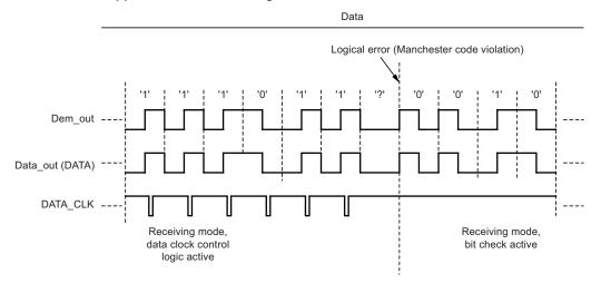
Figure 9-4. Output of the Data Clock After a Successful Bit Check
