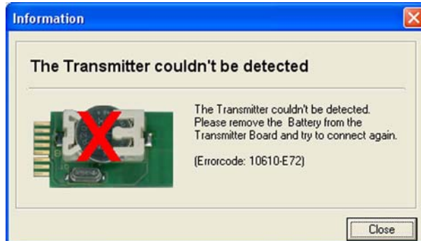
Figure 2-3. Error Code for Removing the Battery during the Programming Process
