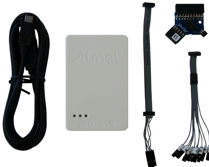
Figure 2-1. Atmel-ICE Full Kit Contents
