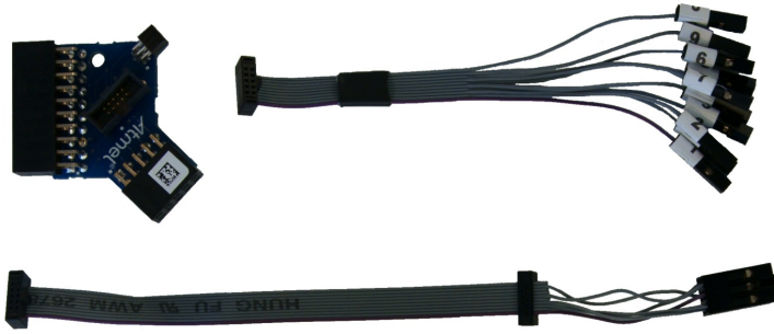
Figure 2-5. Atmel-ICE Cable Kit Contents
