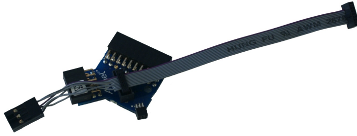
Figure 2-10. Atmel-ICE AVR Probe Connection
