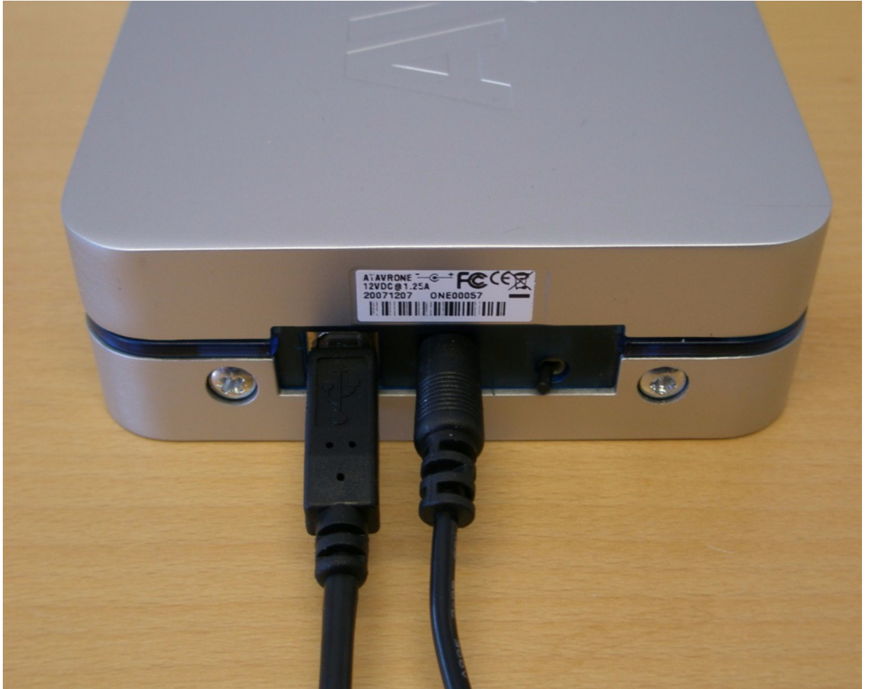
Figure 3-19. AVR ONE! connected to power and USB
