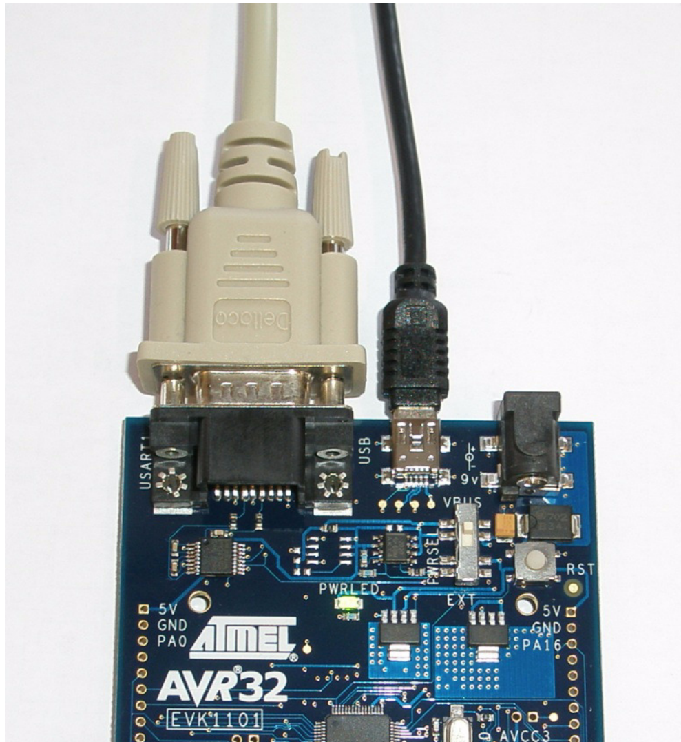
Figure 4-2. Powering the EVK1101 using the USB cable
