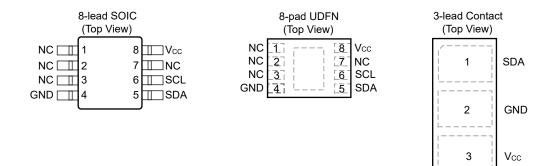
**Note:** The UDFN backside paddle is recommended to be connected to GND.
