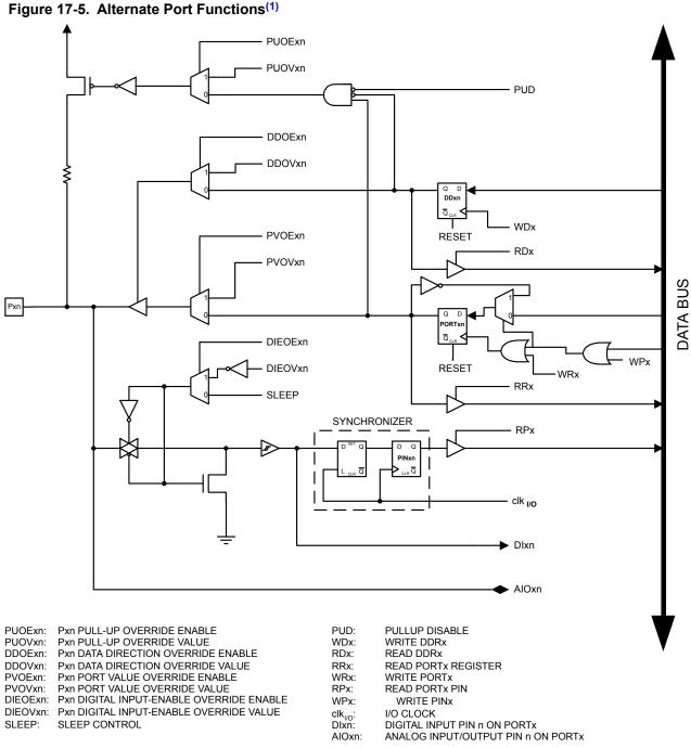
**Note:** 1. WRx, WPx, WDx, RRx, RPx, and RDx are common to all pins within the same port.  $clk_{I/O}$ , SLEEP, and PUD are common to all ports. All other signals are unique for each pin.
