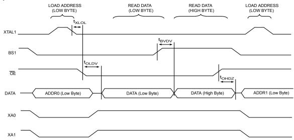
**Note:** The timing requirements shown in Parallel Programming Characteristics (i.e.,  $t_{DVXH}$ ,  $t_{XHXL}$ , and  $t_{XLDX}$ ) also apply to reading operation.
