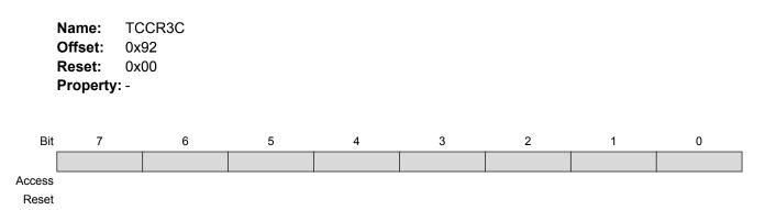
The FOC3A/FOC3B bits are only active when the WGM3[3:0] bits specifies a non-PWM mode. When writing a logical one to the FOC3A/FOC3B bit, an immediate compare match is forced on the Waveform Generation unit. The OC3A/OC3B output is changed according to its COM3x[1:0] bits setting. Note that
