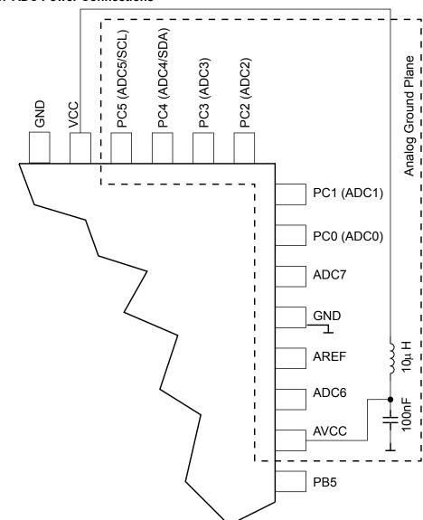
Figure 28-9. ADC Power Connections
