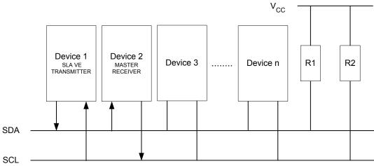
To initiate the SR mode, the TWI (Slave) Address Register (TWARn) and the TWI Control Register (TWCRn) must be initialized as follows:
