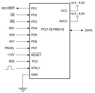
Note: V<sub>CC</sub> - 0.3V < AV<sub>CC</sub> < V<sub>CC</sub> + 0.3V; however, AV<sub>CC</sub> should always be within 4.5 - 5.5V
