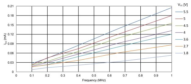
Figure 34-8. ATmega32PB: Idle Supply Current vs. Low Frequency (0.1-1.0MHz)
