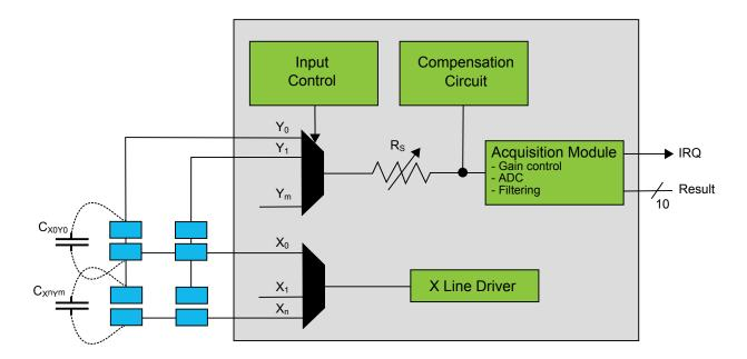
Figure 29-2. PTC Block Diagram Self-Capacitance
