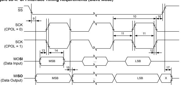
Figure 33-4. SPI Interface Timing Requirements (Slave Mode)
