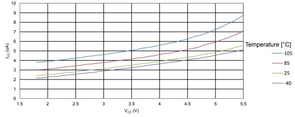
Figure 34-15. ATmega328PB: Power-Down Supply Current vs. V<sub>CC</sub> (AREF, VCCDIV2)
