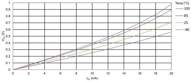
Figure 34-23. ATmega328PB: I/O Pin Output Voltage vs. Sink Current (V<sub>CC</sub> = 5V)
