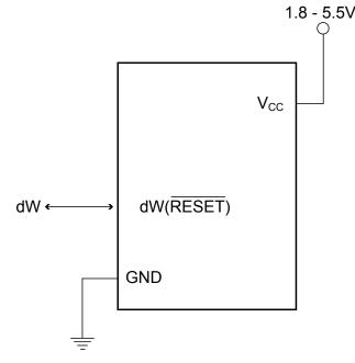
The debugWIRE Setup shows the schematic of a target MCU, with debugWIRE enabled, and the emulator connector. The system clock is not affected by debugWIRE and will always be the clock source selected by the CKSEL Fuses.
