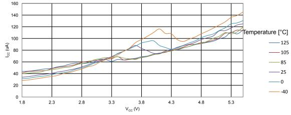
Figure 34-49. ATmega328PB: AREF External Reference Current vs. Vcc
