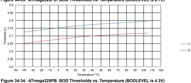
Figure 34-33. ATmega328PB: BOD Thresholds vs. Temperature (BODLEVEL is 2.7V)
