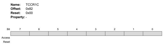
The FOC1A/FOC1B bits are only active when the WGM1[3:0] bits specifies a non-PWM mode. When writing a logical one to the FOC1A/FOC1B bit, an immediate compare match is forced on the Waveform Generation unit. The OC1A/OC1B output is changed according to its COM1x[1:0] bits setting. Note that the FOC1A/FOC1B bits are implemented as strobes. Therefore it is the value present in the COM1x[1:0] bits that determine the effect of the forced compare.
