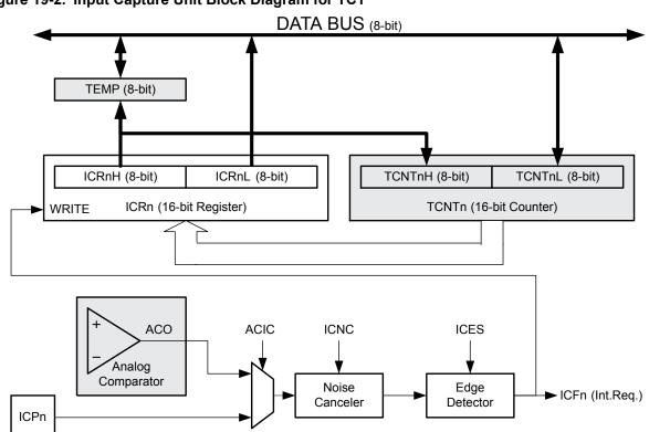
Figure 19-2. Input Capture Unit Block Diagram for TC1
