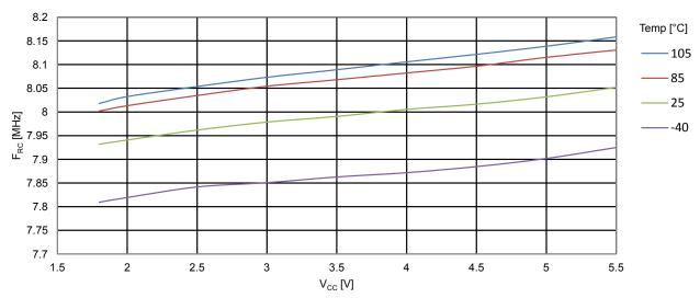
Figure 34-43. ATmega328PB: Calibrated 8MHz RC Oscillator Frequency vs. V<sub>CC</sub>
