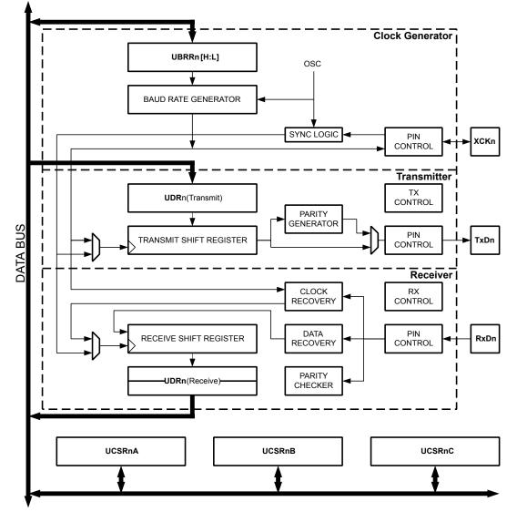
Note: Refer to the Pin Configurations and the I/O-Ports description for USART pin placement.
