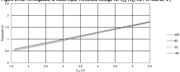
Figure 34-30. ATmega328PB Reset Input Threshold Voltage vs. V<sub>CC</sub> (V<sub>IL</sub>, I/O Pin read as '0')
