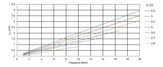
Figure 34-54. ATmega328PB: Reset Supply Current vs. Vcc (Excluding current through Reset Pullup)
