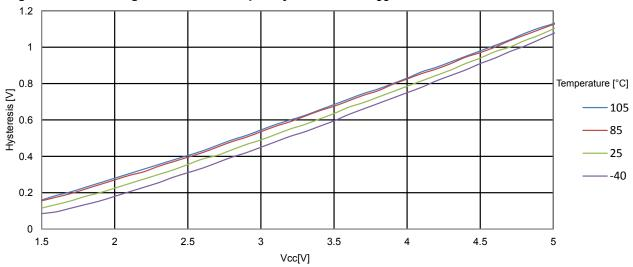
Figure 34-29. ATmega328PB Reset Input Threshold Voltage vs. V<sub>CC</sub> (V<sub>IH</sub>, I/O Pin read as '1')
