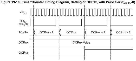
**Note:** The "n" in the register and bit names indicates the device number (n = 1, 3, 4 for Timer/Counter 1, 3, 4), and the "x" indicates Output Compare unit (A/B).
