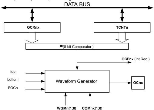
Figure 18-3. Output Compare Unit, Block Diagram
