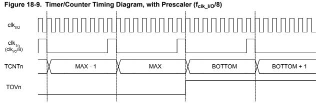
**Note:** The "n" in the register and bit names indicates the device number (n = 0 for Timer/Counter 0), and the "x" indicates Output Compare unit (A/B).
