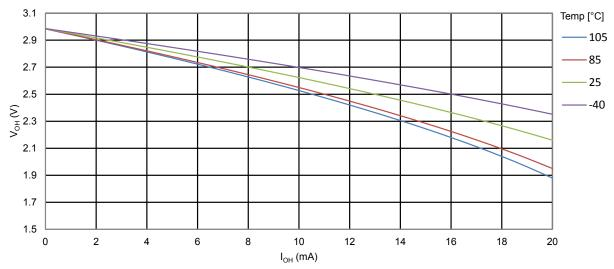
Figure 34-25. ATmega328PB I/O Pin Output Voltage vs. Source Current (V<sub>CC</sub> = 5V)
