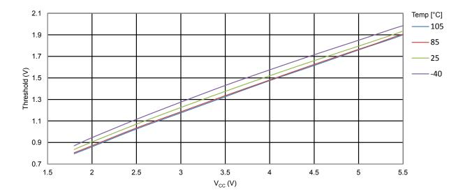
Figure 34-28. ATmega328PB I/O Pin Input Hysteresis vs. V<sub>CC</sub>
