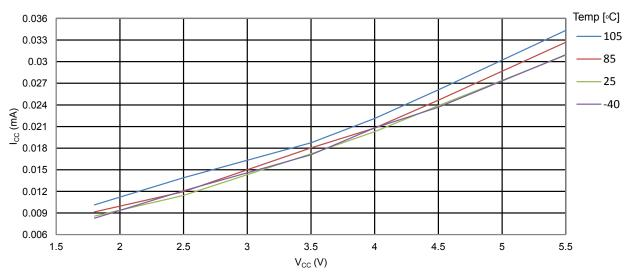
Figure 34-10. ATmega328PB: Idle Supply Current vs. V<sub>CC</sub> (Internal RC Oscillator, 128kHz)
