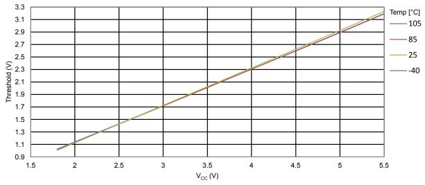
Figure 34-27. ATmega328PB I/O Pin Input Threshold Voltage vs. V<sub>CC</sub> (V<sub>IL</sub>, I/O Pin read as '0')
