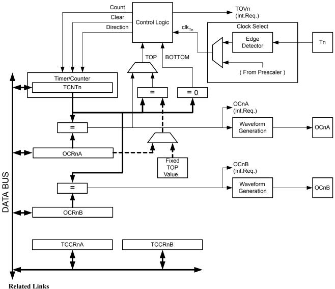
Figure 21-1. 8-bit Timer/Counter Block Diagram
