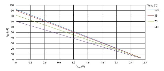
Figure 34-18. ATmega328PB: I/O Pin Pull-up Resistor Current vs. Input Voltage (V<sub>CC</sub> = 5V)
