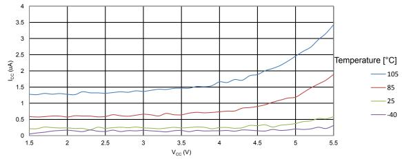
Figure 34-14. ATmega328PB: Power-Down Supply Current vs. V<sub>CC</sub> (Watchdog Timer Enabled)
