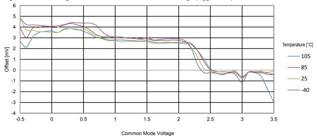
Figure 34-39. ATmega328PB AC Offset vs. Common Voltage (V<sub>CC</sub> = 3.0V)
