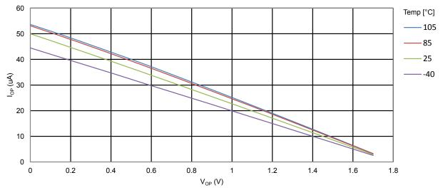
Figure 34-17. ATmega328PB: I/O Pin Pull-up Resistor Current vs. Input Voltage (V<sub>CC</sub> = 2.7V)
