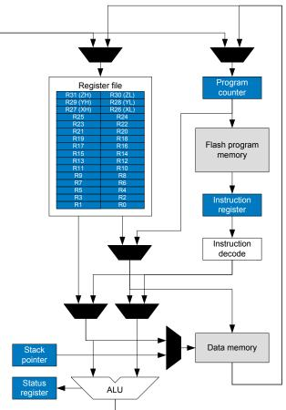
In order to maximize performance and parallelism, the AVR uses a Harvard architecture – with separate memories and buses for program and data. Instructions in the program memory are executed with a single level pipelining. While one instruction is being executed, the next instruction is pre-fetched from the program memory. This concept enables instructions to be executed in every clock cycle. The program memory is In-System Reprogrammable Flash memory.
