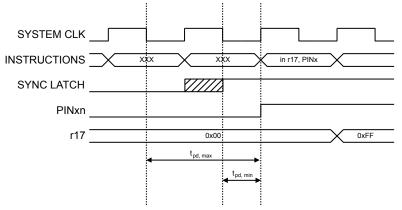
Consider the clock period starting shortly after the first falling edge of the system clock. The latch is closed when the clock is low, and goes transparent when the clock is high, as indicated by the shaded
