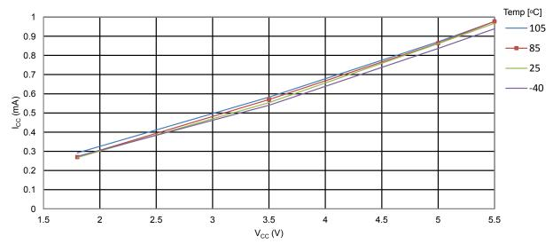
Figure 34-4. ATmega328PB: Active Supply Current vs. V<sub>CC</sub> (Internal RC Oscillator, 1MHz)
