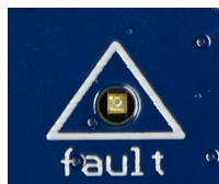
Figure 6-10. Fault LED, used to Indicate the Status of the Analog Sampling Circuitry
