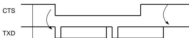
Figure 34-29. Transmitter Behavior when Operating with Hardware Handshaking
