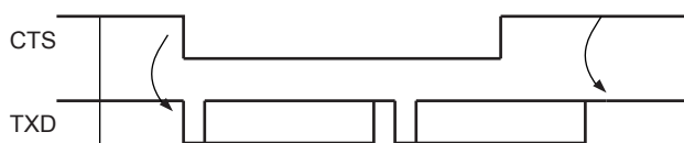
Figure 44-28: Transmitter Behavior when Operating with Hardware Handshaking
