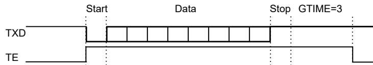
Figure 31-15. Example of TE Drive with Guard Time
