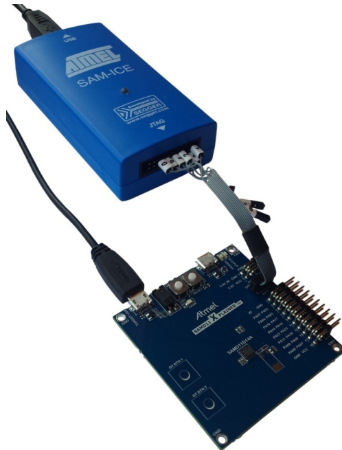
Figure 5-6. SAM-ICE using a Squid Cable
