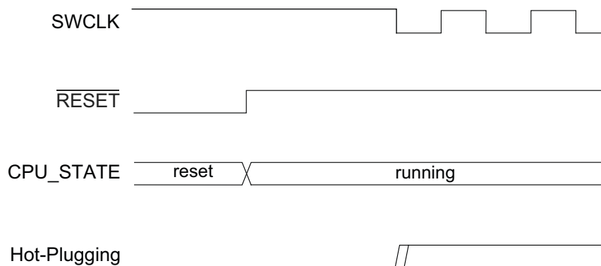
Figure 12-3. Hot-Plugging Detection Timing Diagram
