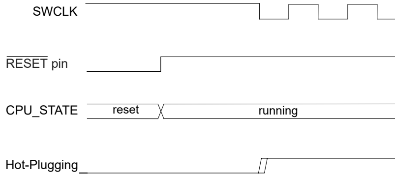
Figure 13-3. Hot-Plugging Detection Timing Diagram
