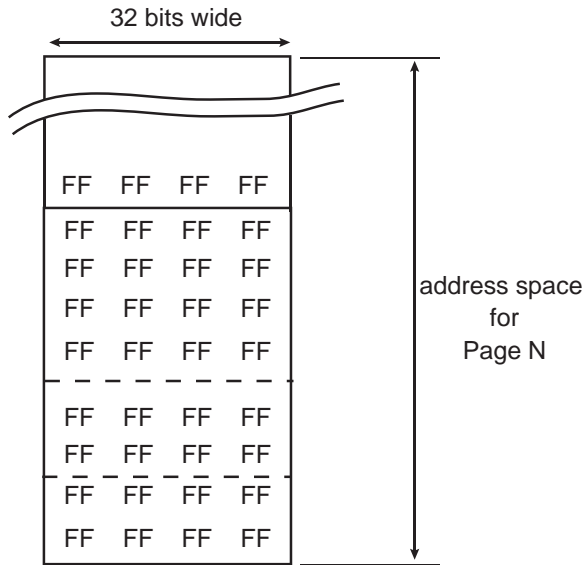
Step 1: Flash array after page erase
