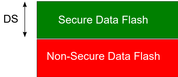
Figure 13-3. SAM L11 Data Flash Memory Mapping
