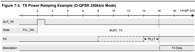
Using an external RF front-end, it may be required to adjust the start-up time of the external PA relative to the internal building blocks to optimize the overall PSD. This can be achieved using the RF\_CTRL\_0.PA\_LT bits.
