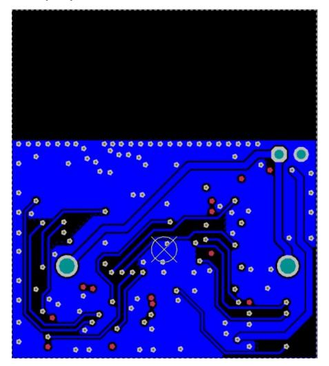
The following figure shows the PCB stack-up for the reference board. Layer 1 (Top layer) and Layer 2 specifications are critical to the RF Trace Layout specification.
