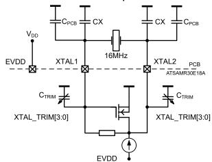
Additional internal trimming capacitors  $C_{TRIM}$  are available. Any value in the range from 0 pF to 4.5 pF with a 0.3 pF resolution is selectable using the XTAL\_TRIM bits in the XOSC\_CTRL register (XOSC\_CTRL.XTAL\_TRIM). To calculate the total load capacitance, the following formula can be used:
