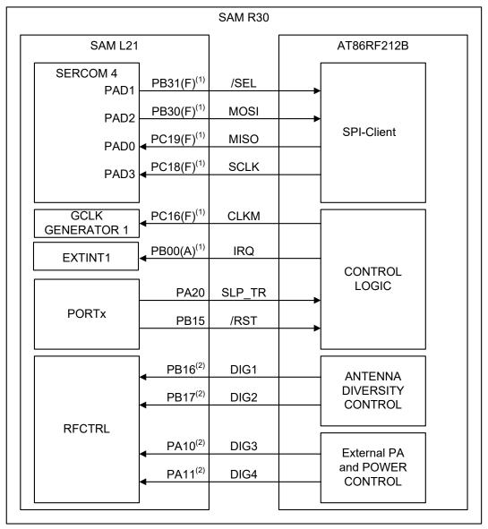
Figure 3-2. Interconnection between SAM L21 and AT86RF212B
