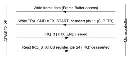
Alternatively, for time critical applications when the frame start transmission time needs to be minimized, a frame transmission task can be started first. Then it can be followed by the Frame Buffer write access event (populating PSDU data). This way the data to be transmitted needs to be written in the transmit frame buffer as the transceiver initializes and begins the SHR transmission.
