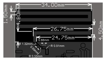
The following figure shows the bottom layer layout of the reference board directly beneath the RF traces.
