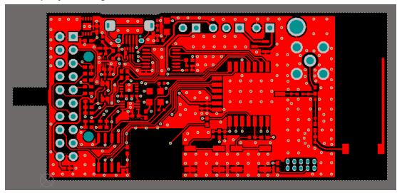
The following figure shows the top layer layout of the reference board focused on the RF traces. The snapshot also indicates the critical dimensions that are required to be replicated in the design to maintain compliance.
