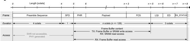
A frame comprises two sections, the radio transceiver internally generated SHR field and the user accessible part stored in the Frame Buffer. The SHR contains the preamble and the SFD field. The variable frame section contains the PHR and the PSDU including the FCS.
