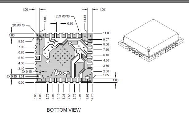
The module can be mounted to a base board with a soldered RF connection.
