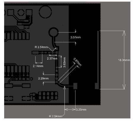
Figure 12-5. Layer 2 (GND) Layout
