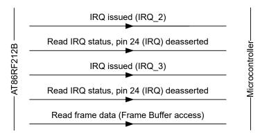
Critical protocol timing could require starting the Frame Buffer read access after interrupt IRQ\_2 (RX\_START). The first byte of the frame data can be read 32µs after the IRQ\_2 (RX\_START) interrupt. The microcontroller must be sure to read slower than the frame is received. Otherwise, a Frame Buffer underrun occurs, IRQ\_6 (TRX\_UR) is issued and the frame data may be not valid. To avoid this, the Frame Buffer read access can be controlled by using a Frame Buffer Empty Indicator.
