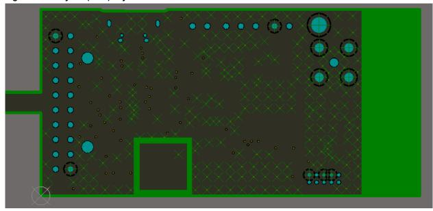
The following figure shows the bottom layer layout of the reference board directly beneath the RF traces.
