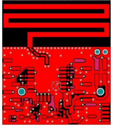
The following figure shows the top layer layout of the reference host Sensor board focussed on RF traces and PCB antenna. The snapshot also indicates the critical dimensions that are required to be replicated in the design to maintain compliance.
