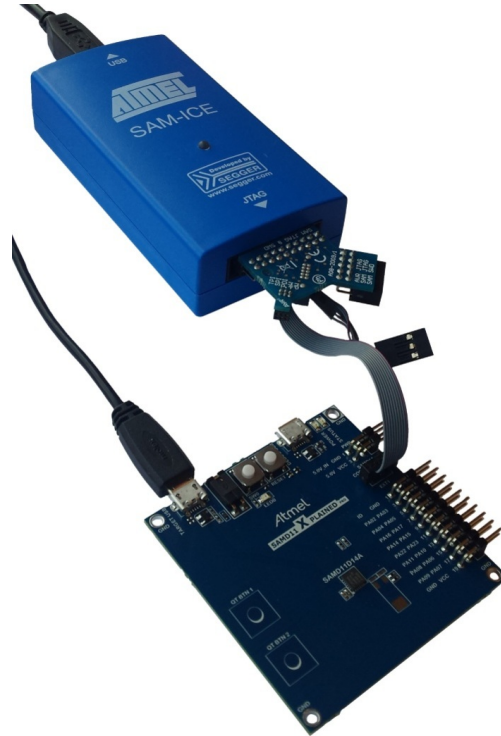
Figure 6-7. SAM-ICE using an Atmel-ICE Adapter
