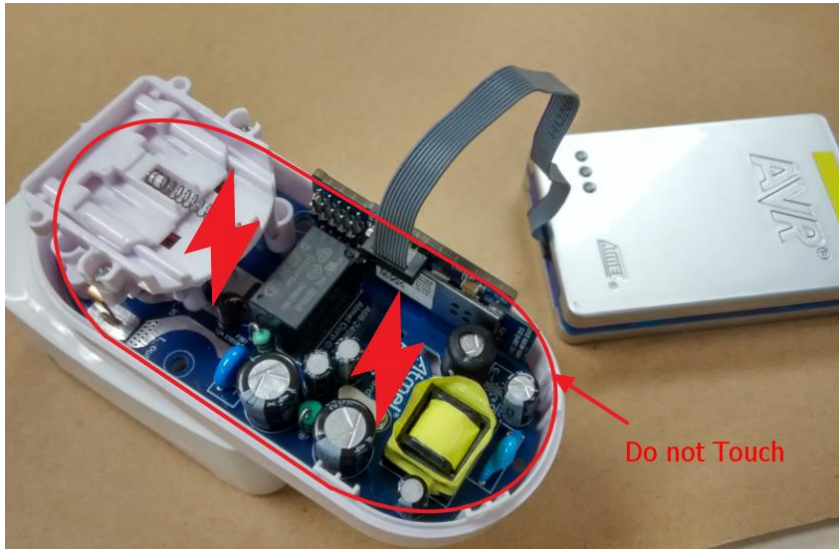
Figure 6-3. Kit Powered by the Onboard AC Input
