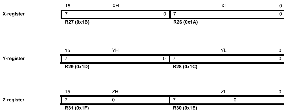
Figure 4-3. The X-, Y-, and Z-registers
