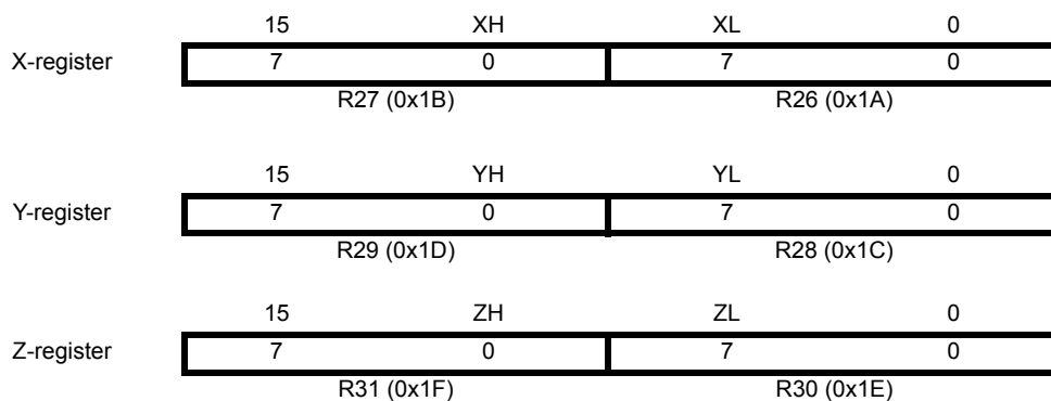
Figure 3-3. The X-, Y-, and Z-registers
