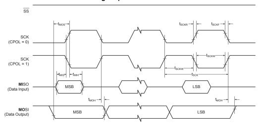
Figure 34-4. USART in SPI Mode - Timing Requirements in Slave Mode
