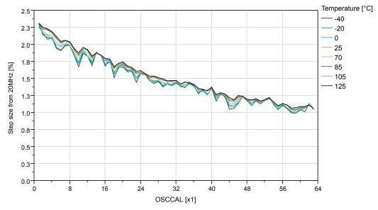
Figure 35-56. OSC20M internal Oscillator: Frequency vs. Calibration Value (V<sub>DD</sub>=3V)
