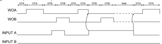
If Input mode 2 is used on input B, an Event will only have an effect if the TCD is in Dead time B or Ontime B, and it will only effect the output WOB.
