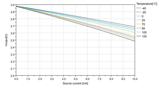
Figure 35-26. IO Pin Output Voltage vs. Source Current (V<sub>DD</sub>=5.0V)
