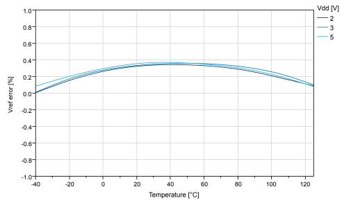
Figure 35-32. Internal 1.1V Reference vs. Temperature
