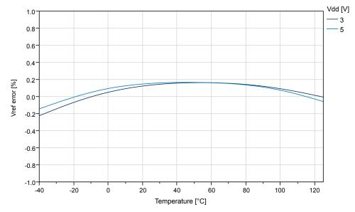
Figure 35-34. Internal 4.3V Reference vs. Temperature
