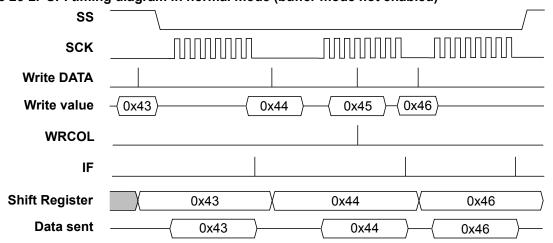
The figure shows three transfers and one write to the DATA register while the SPI is busy with a transfer. This write will be ignored and the Write Collision Flag (INTFLAGS.WRCOL) is set.
