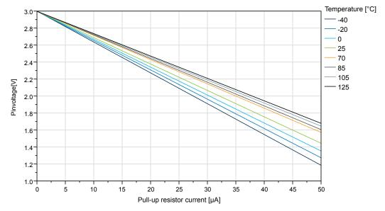
Figure 35-30. IO Pin Pull-Up Resistor Current vs. Input Voltage (V<sub>DD</sub>=5.0V)
