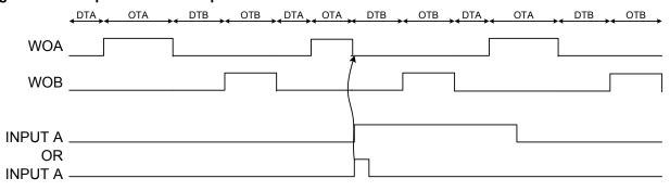
If Input mode 8 is used on input B and an positive input event occurs while in On time B, the TCD counter jumps to Dead time A.
