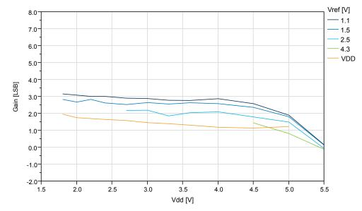
Figure 35-46. Gain Error vs. V<sub>ref</sub> (V<sub>DD</sub>=5.0V, 115ksps)
