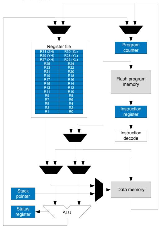
Figure 8-1. AVR CPU Architecture
