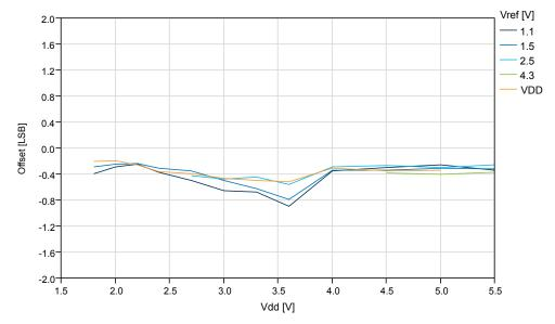
Figure 35-50. Offset Error vs.  $V_{ref}$  ( $V_{DD}$ =5.0V, 115ksps)
