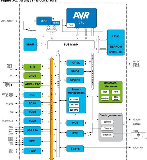
Figure 3-2. ATtiny817 Block Diagram
