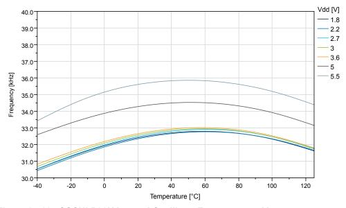
Figure 35-60. OSCULP32K Internal Oscillator Frequency vs. V<sub>DD</sub>
