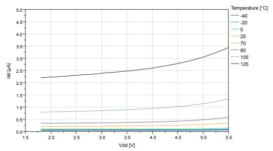
Figure 35-11. Power Down Mode Supply Current vs.  $V_{\rm DD}$  (all functions disabled)
