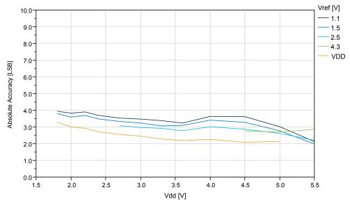
Figure 35-42. Absolute Accuracy vs. V<sub>ref</sub> (V<sub>DD</sub>=5.0V, 115ksps)
