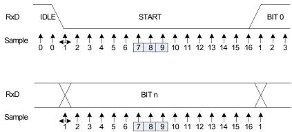
The transmission Baud Rate must be set up in relation to the selected UPDI clock, which can be adjusted by UPDICLKSEL in UPDI.ASI\_CTRLA. See Table 33-2 for recommended maximum and minimum baud rate settings.
