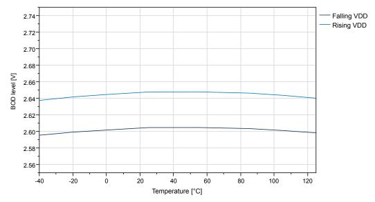
Figure 35-40. BOD Threshold vs. Temperature (Level 4.3V)
