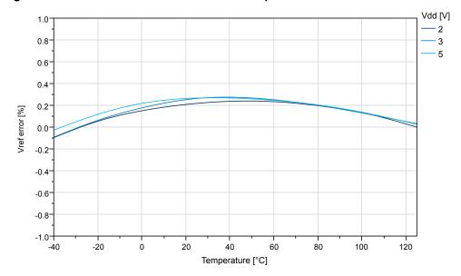
Figure 35-33. Internal 2.5V Reference vs. Temperature
