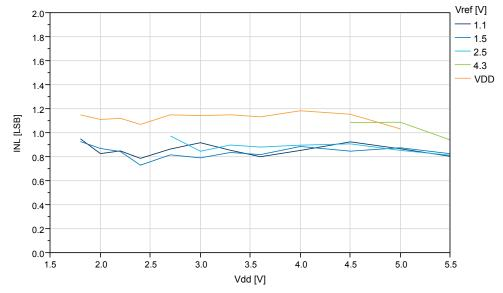
Figure 35-48. INL vs.  $V_{ref}$  ( $V_{DD}$ =5.0V, 115ksps)
