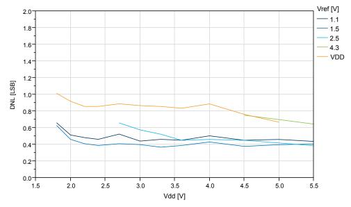
Figure 35-44. DNL vs.  $V_{ref}$  ( $V_{DD}$ =5.0V, 115ksps)
