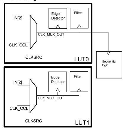
When the Clock Source bit (CLKSRC) is '1', IN[2] is used to clock the corresponding Filter and Edge Detector (CLK\_MUX\_OUT). The Sequential logic is clocked by CLK\_MUX\_OUT of the even LUT in the pair. When CLKSRC bit is '1', IN[2] is treated as MASKed (low) in the TRUTH table.
