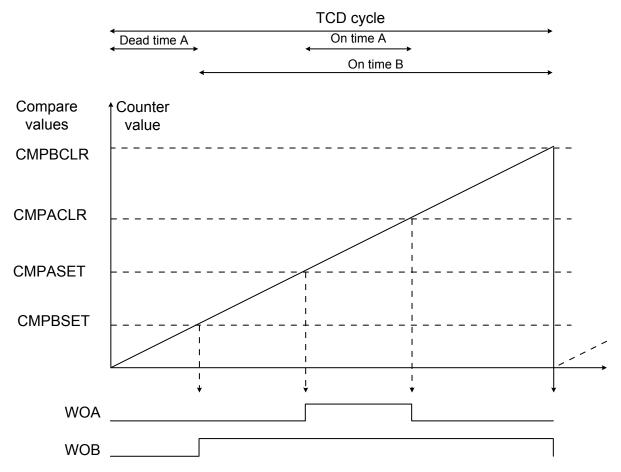
If any of the other compare values are bigger than CMPBCLR it will never be triggered when running in One ramp mode. And if The CMPACLR is smaller than the CMPASET value, the clear value will not have any effect.
