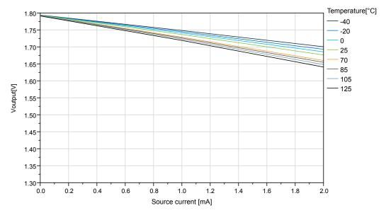
Figure 35-25. IO Pin Output Voltage vs. Source Current (V<sub>DD</sub>=3.0V)
