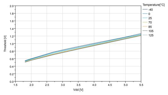
Figure 35-17. IO Pin Input Threshold Voltage vs.  $V_{DD}$  (T=25°C)
