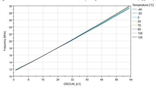
Figure 35-57. OSC20M Internal Oscillator: Frequency vs. Temperature
