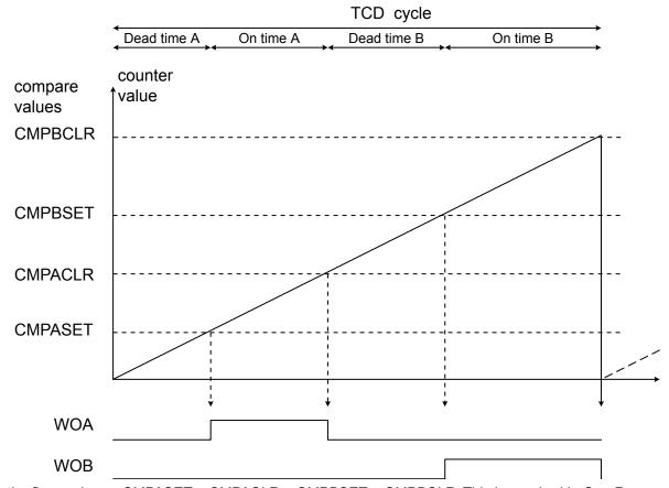
In the figure above, CMPASET < CMPACLR < CMPBSET < CMPBCLR. This is required in One Ramp Mode to avoid overlapping outputs. The figure below is an example where CMPBSET < CMPACLR < CMPBCLR, resulting in an overlap of the outputs.
