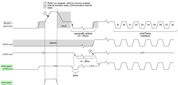
Figure 33-6. UPDI Enable Sequence by 12V Programming
