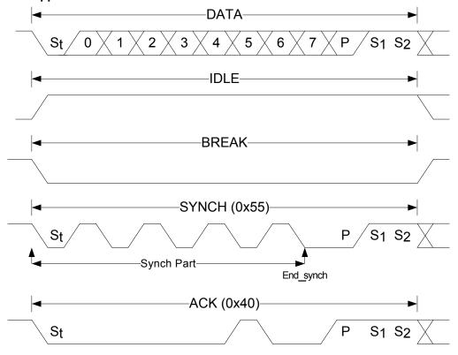
Data Frame Consist of 1 start bit (always low), 8 data bits, 1 parity bit (even parity) and two stop bits (always high). If the start bit, parity bit or stop bits have an incorrect value, an error will be detected and signalized by the UPDI. The parity bit check in the UPDI can be disabled by writing the PARD bit in UPDI.CTRLA, in which case the parity generation from the debugger can be ignored.
