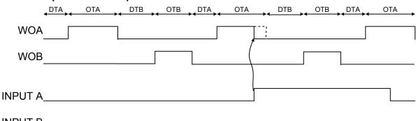
If Input mode 9 is used on input B and an positive input event occurs while in On time B, the output will be off for the rest of the on-time.
