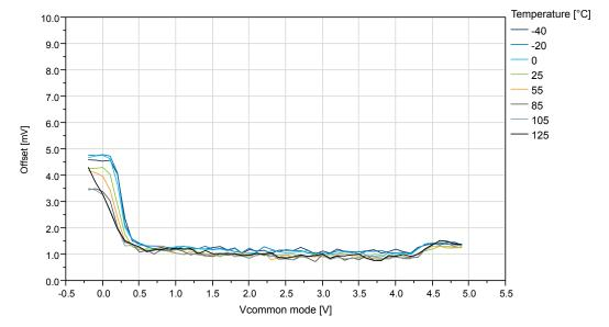
Figure 35-54. Offset vs.  $V_{CM}$  - 10mV to 50mV ( $V_{DD}$ =5V, T=25°C)
