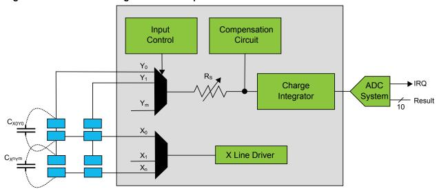
Figure 32-2. PTC Block Diagram Self-Capacitance
