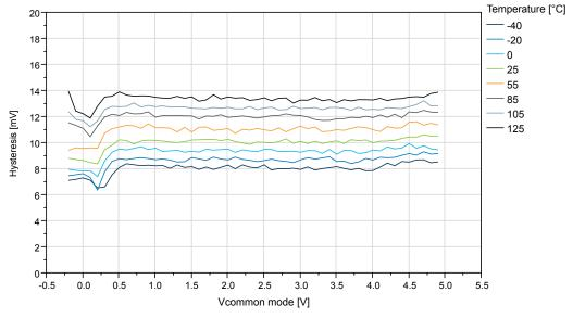
Figure 35-52. Hysteresis vs.  $V_{CM}$  - 10mV to 50mV ( $V_{DD}$ =5V, T=25°C)
