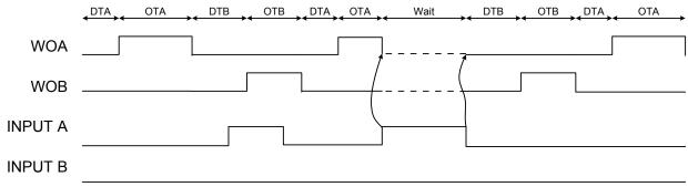
If Input mode 1 is used on input B, an Event will only have an effect if the TCD is in Dead time B or Ontime B, and it will only effect the output WOB. When the event is done, the TCD counter starts at Dead time A.
