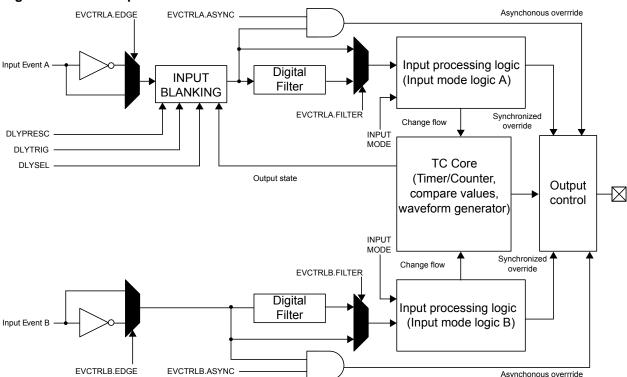
There is a delay of 2-3 clock cycles on the TCD synchronizer clock between receiving the input Event and processing it and overriding the outputs. If using the asynchronous Event detection, the outputs will override instantly outside the input processing.
