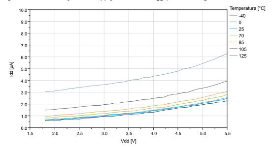
Figure 35-14. : Standby Mode Supply Current vs. V<sub>DD</sub> (Sampled BOD running at 125Hz)
