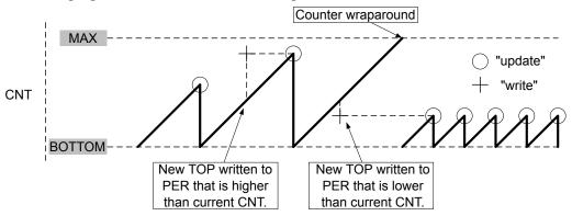
A counter wraparound can occur in any mode of operation when up-counting without buffering. This is due to the fact that the registers TCA.CNT and TCA.PER are continuously compared: if a new TOP value is written to TCA.PER that is lower than current TCA.CNT, the counter will wrap first before a compare match happened.
