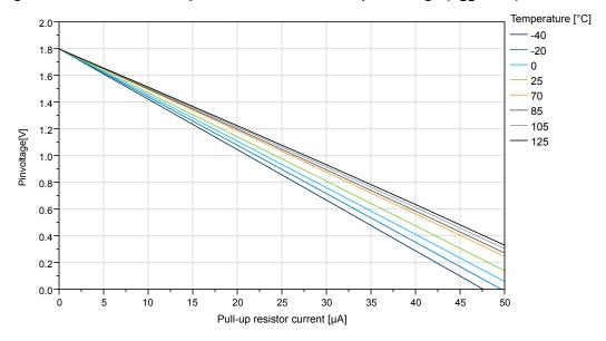
Figure 35-29. IO Pin Pull-Up Resistor Current vs. Input Voltage ( $V_{DD}$ =3.0V)
