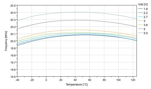
Figure 35-58. OSC20M Internal Oscillator: Frequency vs.  $V_{DD}$
