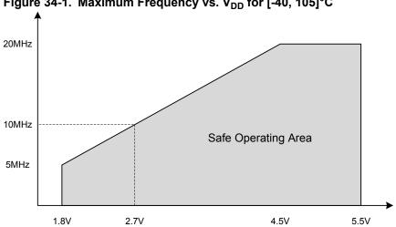
Figure 34-1. Maximum Frequency vs. V<sub>DD</sub> for [-40, 105]°C
