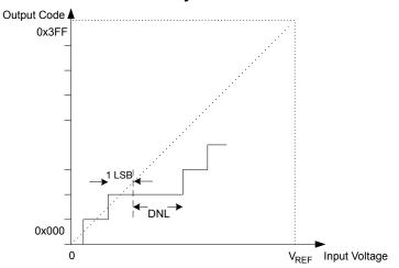
Quantization Error Due to the quantization of the input voltage into a finite number of codes, a range
