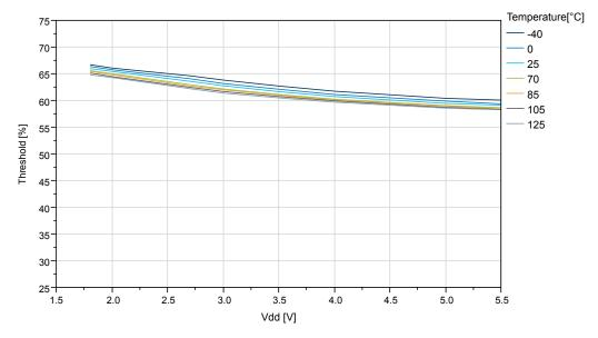
Figure 35-19. IO Pin Input Threshold Voltage vs.  $V_{DD} (V_{IL})$
