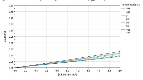
Figure 35-21. IO Pin Output Voltage vs. Sink Current (V<sub>DD</sub>=3.0V)
