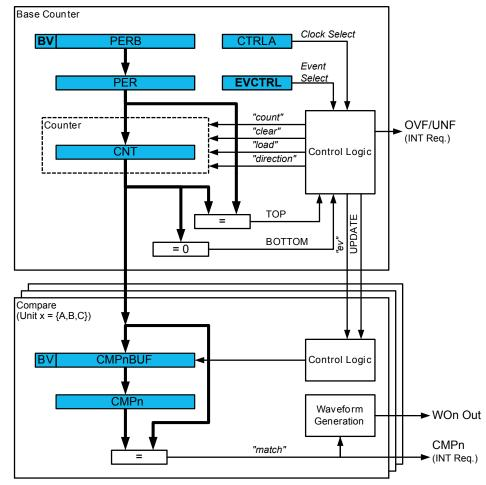
Figure 20-2. Timer/Counter Block Diagram
