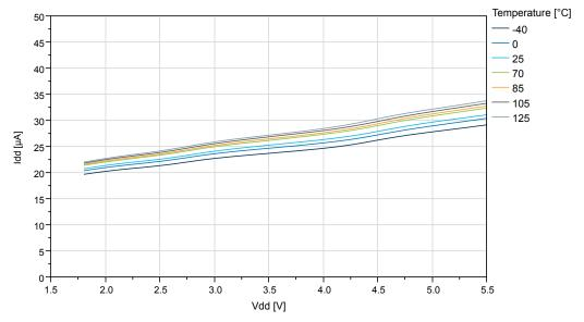
Figure 35-36. BOD Current vs. V<sub>DD</sub> (Sampled BOD at 125Hz)
