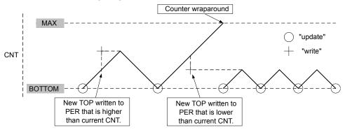
**With Buffering:** When double buffering is used, the buffer can be written at any time and still maintain correct operation. The TCA.PER is always updated on the UPDATE condition, as shown for dual-slope operation in the figure below. This prevents wraparound and the generation of odd waveforms.
