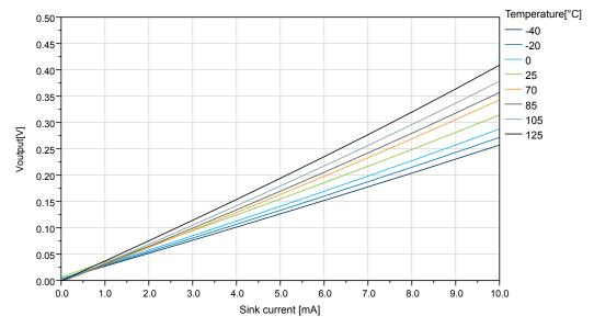
Figure 35-22. IO Pin Output Voltage vs. Sink Current (V<sub>DD</sub>=5.0V)
