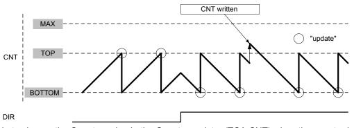
It is possible to change the Counter value in the Counter register (TCA.CNT) when the counter is running. The write access to TCA.CNT has higher priority than count, clear, or reload, and will be immediate. The direction of the counter can also be changed during normal operation by writing to DIR in TCA.CTRLE.
