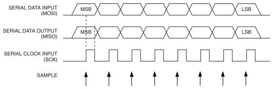
**Table 20-12.** Serial Programming Characteristics,  $T_A = -40^{\circ}\text{C}$  to  $+85^{\circ}\text{C}$ ,  $V_{CC} = 1.8 - 5.5\text{V}$  (Unless Otherwise Noted)
