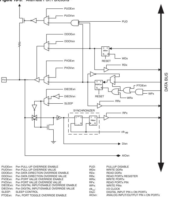
Figure 10-5. Alternate Port Functions<sup>(1)</sup>
