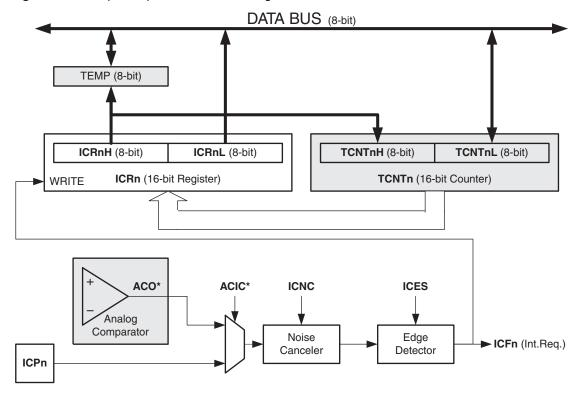
Figure 12-3. Input Capture Unit Block Diagram
