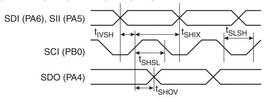
**Table 20-13.** High-voltage Serial Programming Characteristics  $T_A = 25$ °C,  $V_{CC} = 5V$  (Unless otherwise noted)
