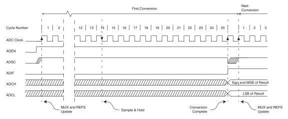
The actual sample-and-hold takes place 1.5 ADC clock cycles after the start of a normal conversion and 13.5 ADC clock cycles after the start of an first conversion. When a conversion is complete, the result is written to the ADC Data Registers, and ADIF is set. In Single Conversion mode, ADSC is cleared simultaneously. The software may then set ADSC again, and a new conversion will be initiated on the first rising ADC clock edge.
