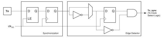
The edge detector generates one  $clk_{T0}$  pulse for each positive (CSn2:0 = 7) or negative (CSn2:0 = 6) edge it detects. The synchronization and edge detector logic introduces a delay of 2.5 to 3.5 system clock cycles from an edge has been applied to the Tn pin to the counter is updated.
