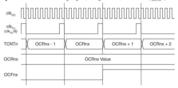
Figure 12-12 on page 104 shows the count sequence close to TOP in various modes. When using phase and frequency correct PWM mode the OCR1x Register is updated at BOTTOM. The timing diagrams will be the same, but TOP should be replaced by BOTTOM, TOP-1 by BOTTOM+1 and so on. The same renaming applies for modes that set the TOV1 flag at BOTTOM.
