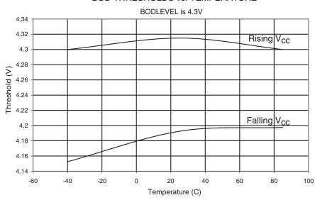
BOD THRESHOLDS vs. TEMPERATURE
