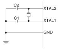
C1 and C2 should always be equal for both crystals and resonators. The optimal value of the capacitors depends on the crystal or resonator in use, the amount of stray capacitance, and the electromagnetic noise of the environment. Some initial guidelines for choosing capacitors for use with crystals are given in Table 6-9 below. For ceramic resonators, the capacitor values given by the manufacturer should be used.
