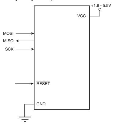
Note: If clocked by internal oscillator there is no need to connect a clock source to the CLKI pin.
