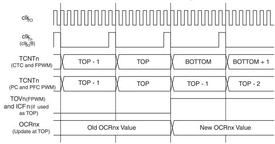
Figure 12-13. Timer/Counter Timing Diagram, with Prescaler (f<sub>clk I/O</sub>/8)
