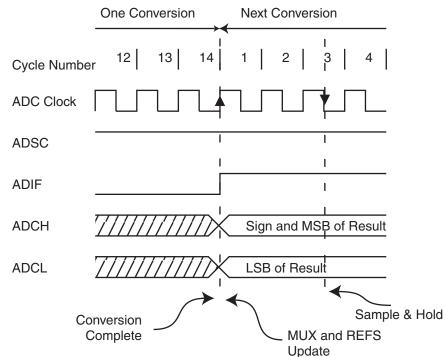
Figure 16-7. ADC Timing Diagram, Free Running Conversion
