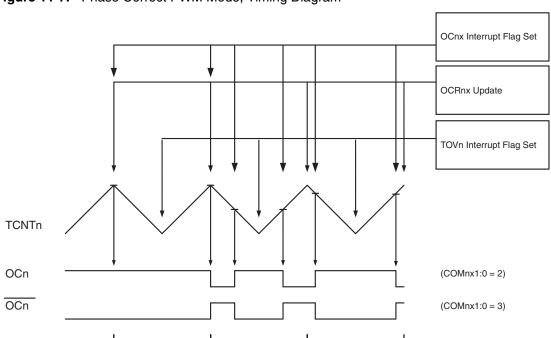
Figure 11-7. Phase Correct PWM Mode, Timing Diagram
