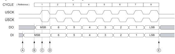
Figure 14-3. Three-wire Mode, Timing Diagram
