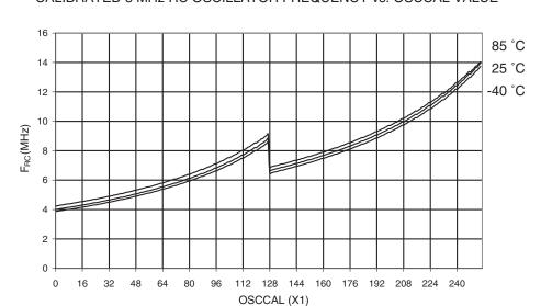
Figure 21-42. Calibrated 8 MHz RC Oscillator Frequency vs. OSCCAL Value
