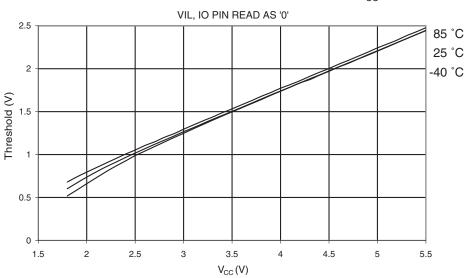
I/O PIN INPUT THRESHOLD VOLTAGE vs. V<sub>CC</sub>
