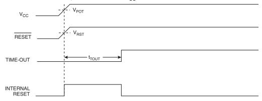
Figure 8-3. MCU Start-up, RESET Extended Externally
