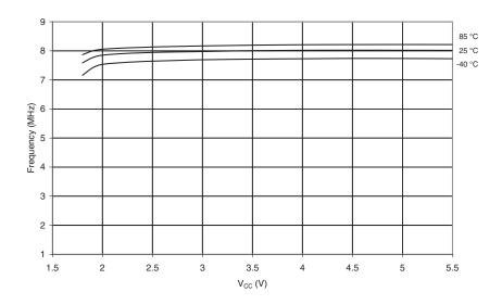
Figure 21-41. Calibrated 8 MHz RC oscillator Frequency vs. Temperature
