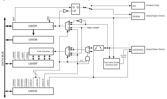
The 8-bit USI Data Register (USIDR) contains the incoming and outgoing data. It is directly accessible via the data bus but a copy of the contents is also placed in the USI Buffer Register (USIBR) where it can be retrieved later. If reading the USI Data Register directly, the register must be read as quickly as possible to ensure that no data is lost.
