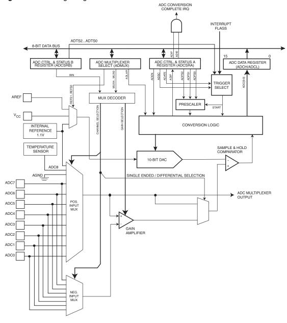
Figure 16-1. Analog to Digital Converter Block Schematic
