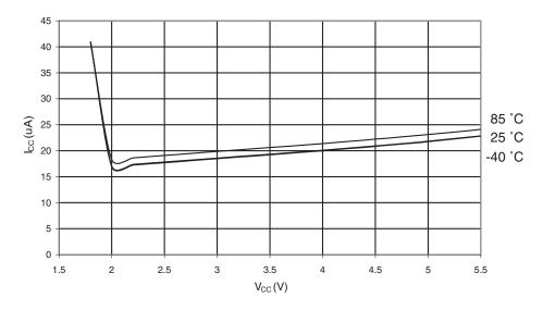
Figure 21-50. Watchdog Timer Current vs.  $V_{CC}$  WATCHDOG TIMER CURRENT vs.  $V_{CC}$
