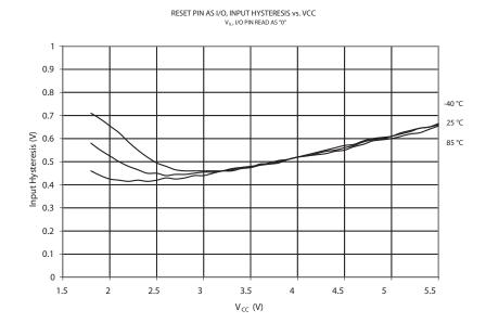
Figure 21-34. Reset Pin Input Hysteresis vs.  $V_{CC}$  (Reset Pin Used as I/O)
