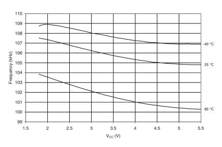
Figure 21-39. Watchdog Oscillator Frequency vs. Temperature
