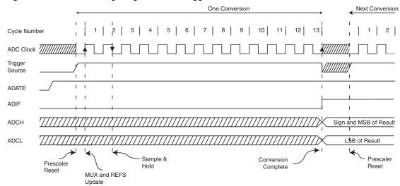
Figure 16-6. ADC Timing Diagram, Auto Triggered Conversion
