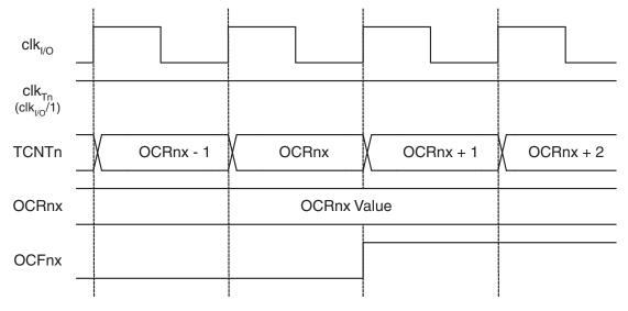
Figure 12-11 on page 104 shows the same timing data, but with the prescaler enabled.
