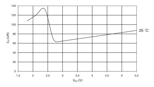
Figure 21-46. Programming Current vs.  $V_{\text{CC}}$  (ATtiny24)
