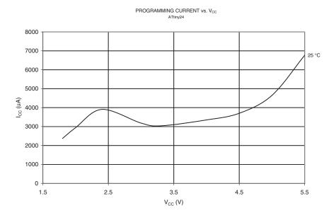
Figure 21-47. Programming Current vs. V<sub>CC</sub> (ATtiny44)
