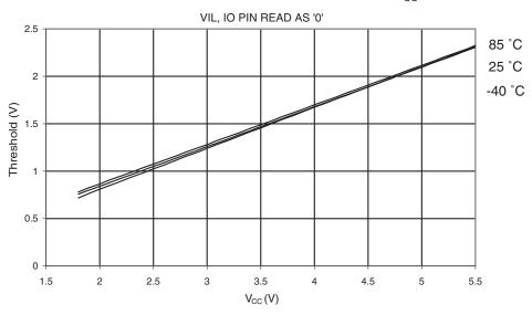
Figure 21-33. Reset Pin Input Hysteresis vs.  $V_{\rm CC}$
