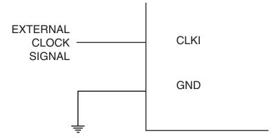
When this clock source is selected, start-up times are determined by the SUT Fuses as shown in Table 6-3.
