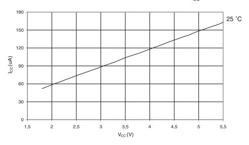
Figure 21-45. Analog Comparator Current vs. V<sub>CC</sub>
