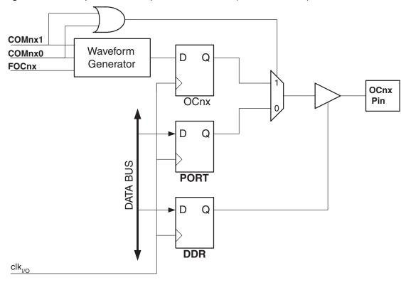
Figure 12-5. Compare Match Output Unit, Schematic (non-PWM Mode)
