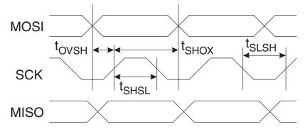
Figure 20-5. Serial Programming Waveform
