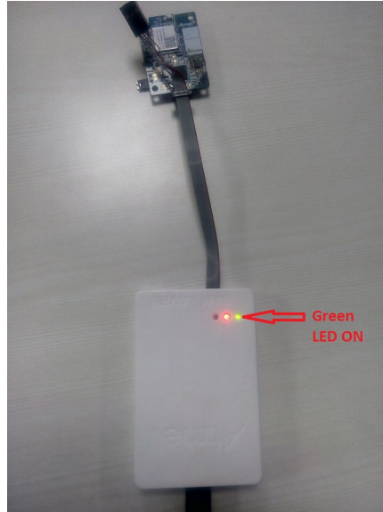
Figure 3-4. Atmel-ICE 10-pin Header Orientation
