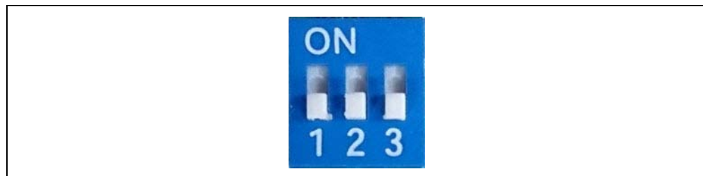
FIGURE 3-35: SWITCH SW9 IN FLASH APPLICATION MODE
