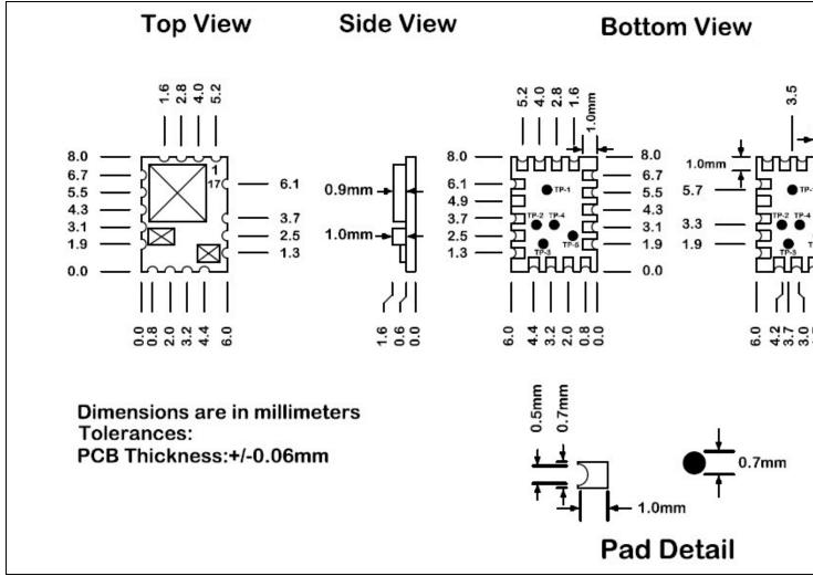
Figure 6-8 illustrates the recommended PCB footprint.
