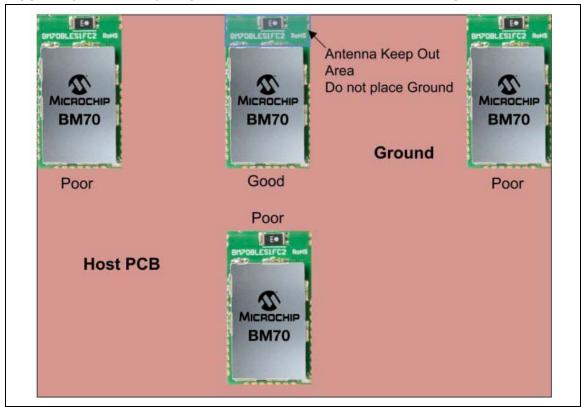
Figure 4-4 illustrates a typical example of good and poor antenna placement of the BM71BLES1FC2 module on the main application board with the ground plane.
