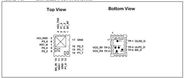
FIGURE 1-6: BM71BLES1FC2 PIN DIAGRAM
