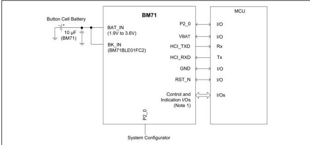
**Note 1:** Hardware functions can include ADC and PWM. Refer to "BM70/71 Bluetooth® Low Energy Module User's Guide" (DS50002542) for a full description of all possible configurable behavior and hardware.
