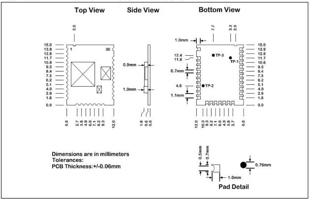
Figure 6-4 illustrates the recommended PCB footprint.
