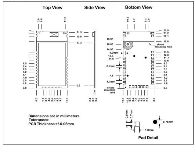
Figure 6-2 illustrates the recommended PCB footprint. Ensure that no top copper layer is near the test pin area.
