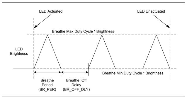
Figure 6.6 Breathe Behavior with Inverted Polarity
