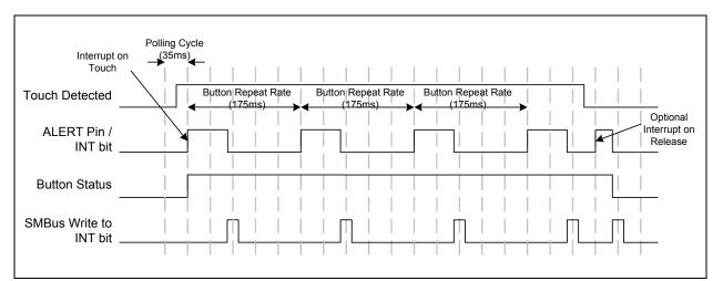
Figure 5.2 Button Interrupt Behavior - Repeat Rate Enabled
