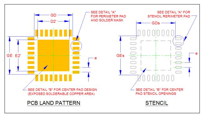
Figure 7.3 Package PCB Land Pattern and Stencil
