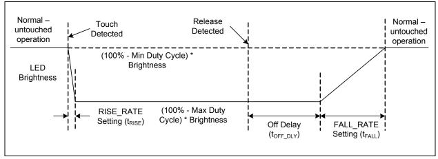
Figure 6.7 Direct Behavior for Non-Inverted Polarity
