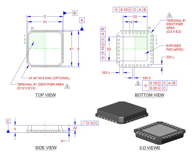
Figure 7.1 Package Diagram - 32-Pin QFN
