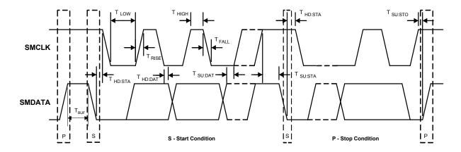
Figure 4.1 SMBus Timing Diagram
