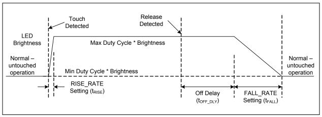
Figure 6.8 Direct Behavior for Inverted Polarity
