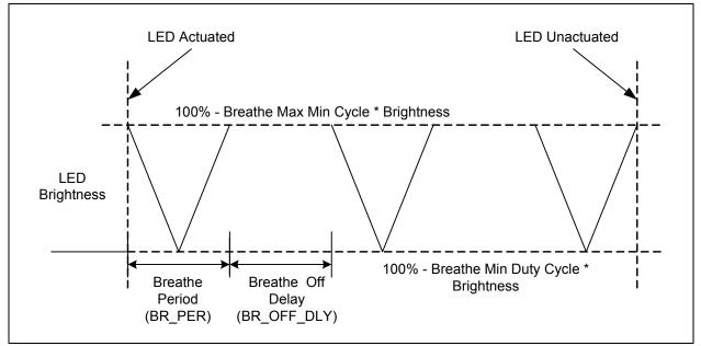
Figure 6.5 Breathe Behavior with Non-Inverted Polarity
