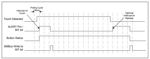
Figure 5.3 Button Interrupt Behavior - No Repeat Rate Enabled
