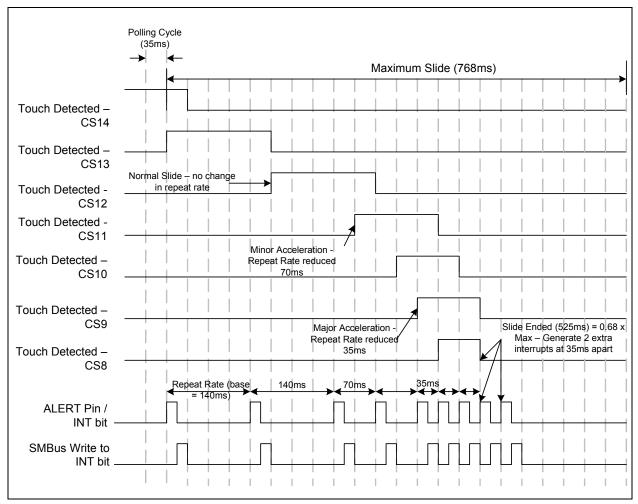
Figure 5.7 Slide Interrupt Behavior - Acceleration Example
