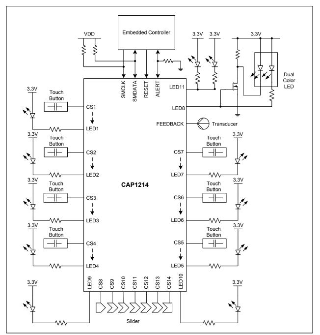
Figure 5.1 System Diagram for CAP1214
