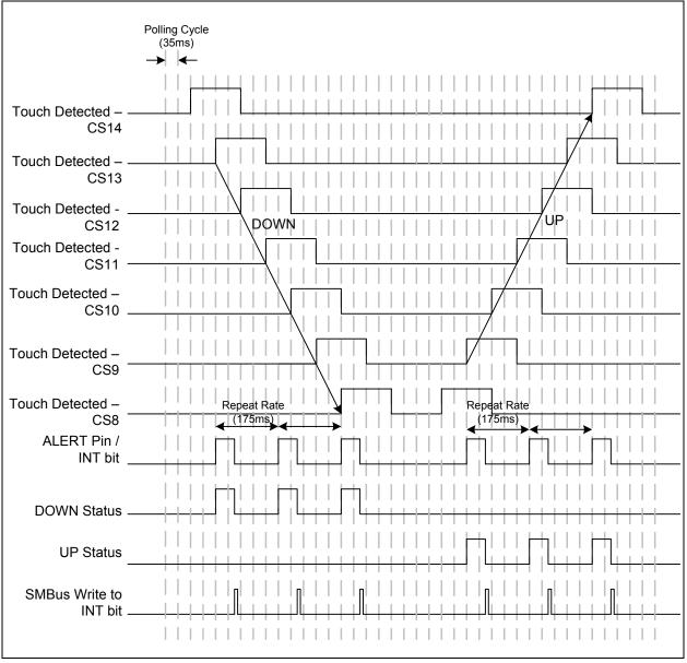
Figure 5.6 Slide Interrupt Behavior - No Acceleration
