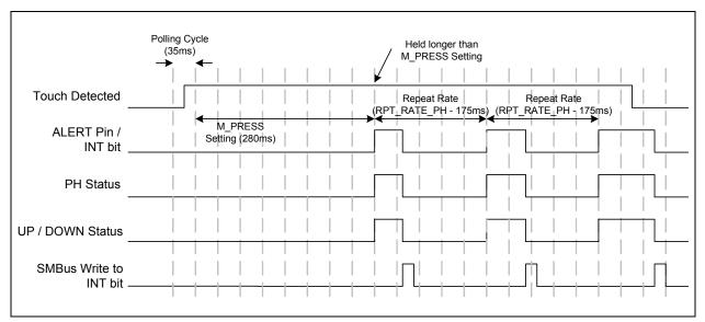
Figure 5.5 Press and Hold Interrupt Behavior
