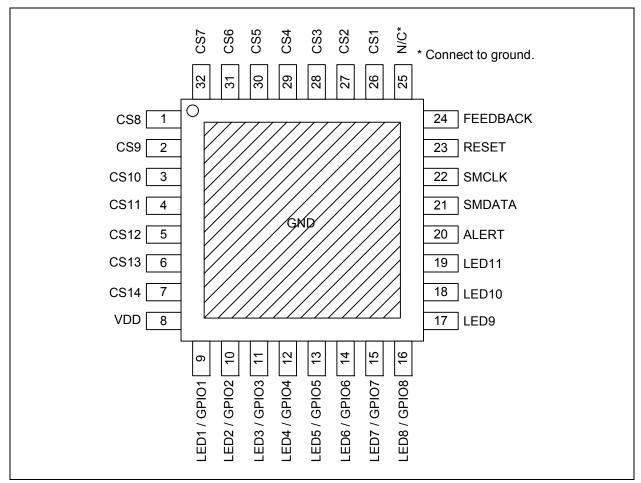
Figure 1.1 CAP1214 Pin Diagram (32-Pin QFN)
