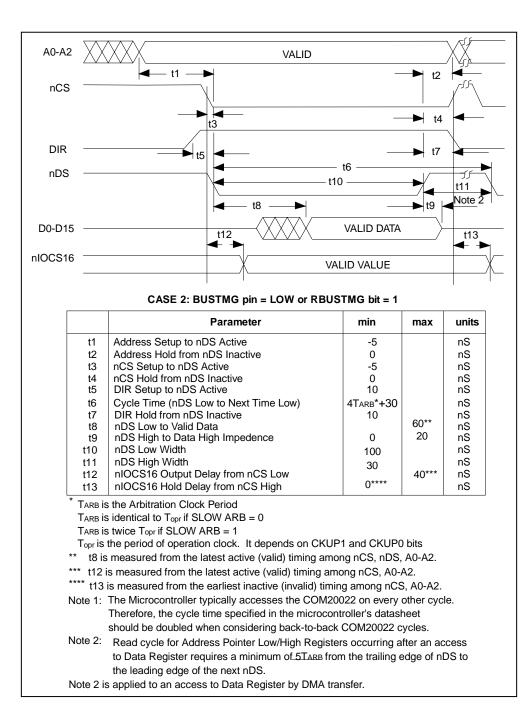
Figure 8.8 - Non-Multiplexed Bus, 68XX-Like Control Signals; Read Cycle
