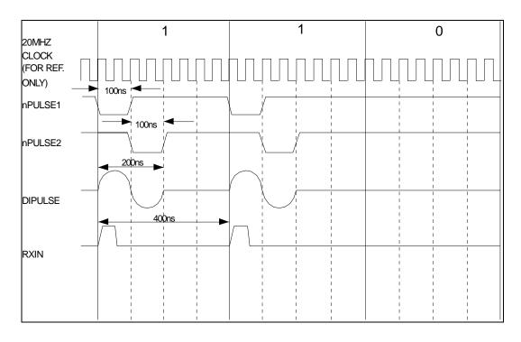
Figure 5.9 - Dipulse Waveform for Data of 1-1-0
