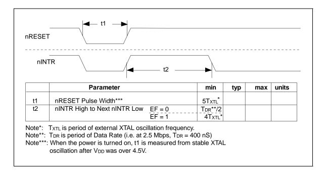
Figure 8.16 - Reset and Interrupt Timing
