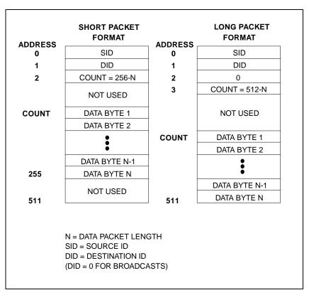
Figure 6.3 - RAM Buffer Packet Configuration
