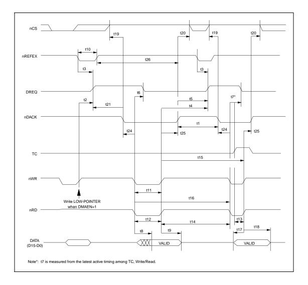
Figure 8.17 - DMA Timing (Intel Mode 80XX)
