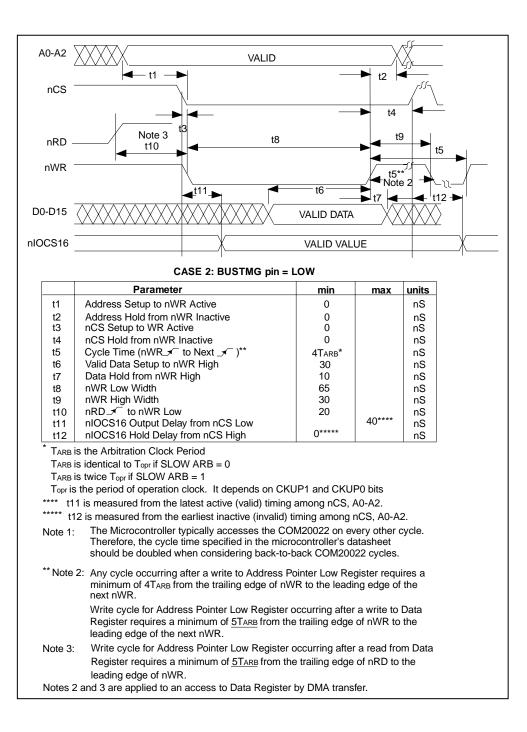
Figure 8.10 - Non-Multiplexed Bus, 80XX-Like Control Signals; Write Cycle
