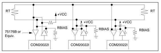
Figure 5.8 - COM20022I Network Using RS-485 Differential Transceivers
