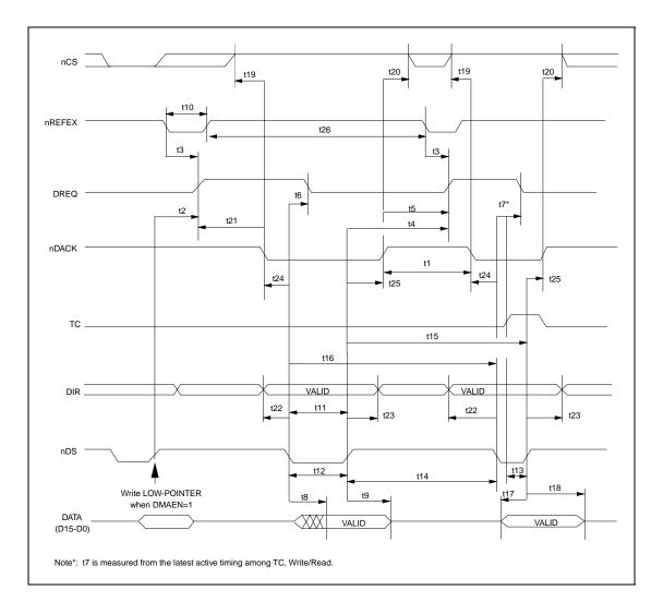
Figure 8.18 - DMA Timing (Motorola Mode 68XX)
