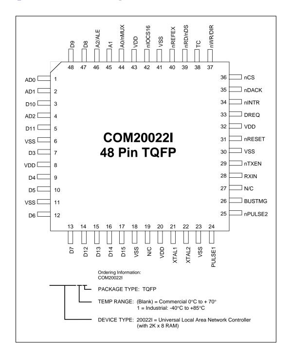
Figure 2.1 - COM20022I Pin Configuration
