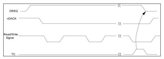
Figure 5.6 - Burst Mode DMA Data Transfer Rough Timing
