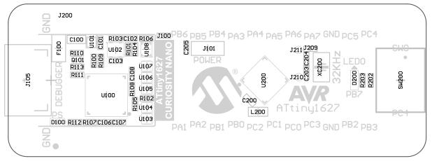
Figure 7-3. ATtiny1627 Curiosity Nano Assembly Drawing Bottom
