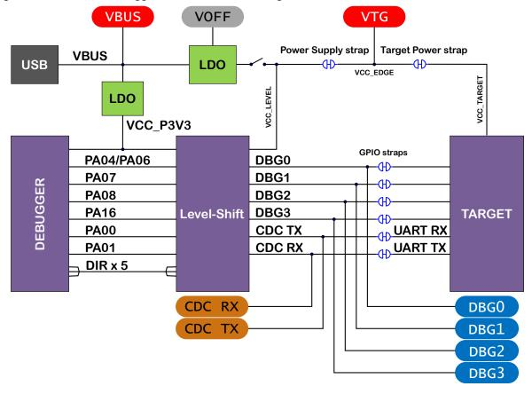
Figure 7-5. On-Board Debugger Connections Block Diagram
