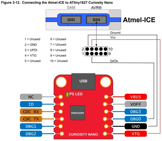
To avoid contention between the external debugger and the on-board debugger, do not start any programming/debug operation with the on-board debugger through Atmel Studio/Microchip MPLAB® X IDE or mass storage programming while the external tool is active.
