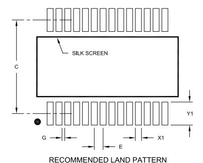
Units MILLIMETERS MIN MOM MAX **Dimension Limits** Contact Pitch 0.65 BSC Ε Contact Pad Spacing С 7.20 Contact Pad Width (X28) Χ1 0.45 Contact Pad Length (X28) Y1 1.75 Distance Between Pads G 0.20
