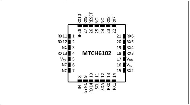
FIGURE 2-2: 28-PIN SSOP
