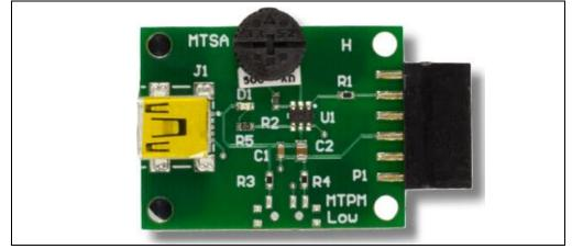
Figure 1-3 shows the Controller board with the MTCH101 chip (U1 Chip on board). It is responsible for the touch event detection, its processing, and its output by lighting the red LED (D1). It expects a capacitive touch sensor on the female 12-pin header connector to the right of the chip. The Proximity sensor board included in the package can be connected or the user can connect one sensor to pin 2 of the 12-pin header connector.
