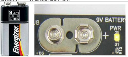
The PICDEM 2 Plus Demonstration Board can be powered with an external 9V battery for a power supply.
