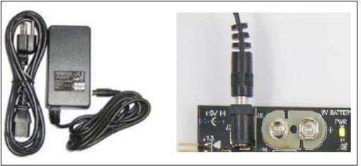
The PICDEM 2 Plus Demonstration Board can be powered with an external 9V power supply.
