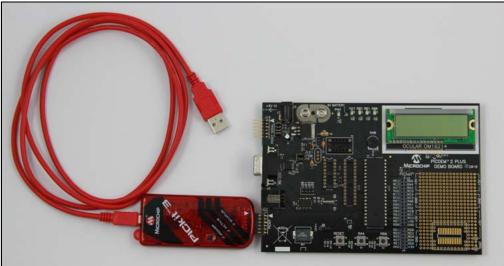
Microchip's PICkit 3 In-Circuit Debugger/Programmer uses in-circuit debugging logic incorporated into each chip with Flash memory to provide a low-cost hardware debugger and programmer.
