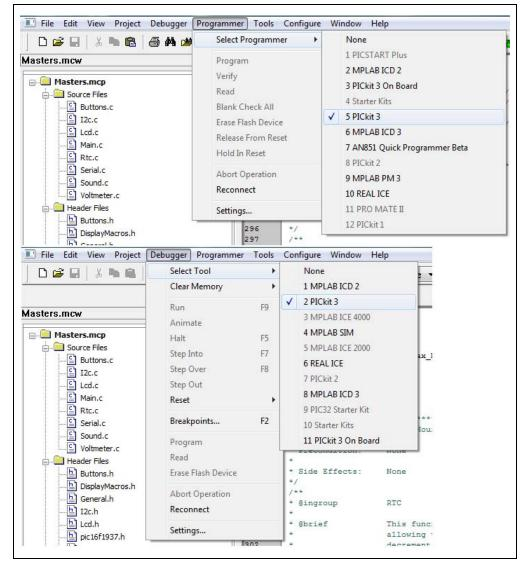
FIGURE 2-2: CONNECTING A PICkit PROGRAMMER
