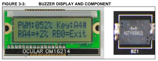
This mode turns on the Piezo buzzer using the CCP1 module I/O pin, RC2.
