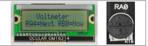
This mode uses the A/D module to measure the voltage of the RA0 pot (R16) and display a voltage between 0.00V and 5.00V on the LCD.
