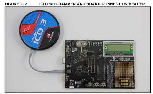
The MPLAB<sup>®</sup> ICD 3 In-Circuit Debugger System is Microchip's most cost-effective, high-speed hardware debugger/programmer for Microchip Flash Digital Signal Controller (DSC) and microcontroller (MCU) devices. It debugs and programs PIC<sup>®</sup> Flash microcontrollers and dsPIC<sup>®</sup> DSCs with the powerful, yet easy-to-use graphical user interface of MPLAB Integrated Development Environment (IDE).
