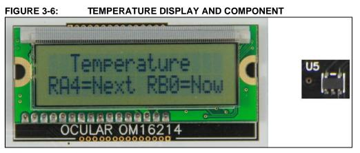
This mode uses a TC74 thermal sensor to measure ambient temperature in Celsius and then display the temperature on the LCD. The user has the option to change the display between Celsius and Fahrenheit by pressing RB4.
