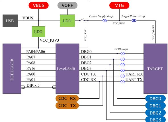
Figure 7-6. On-Board Debugger Connection Cut Straps
