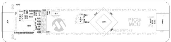
Figure 7-3. PIC18F57Q43 Curiosity Nano Assembly Drawing Bottom
