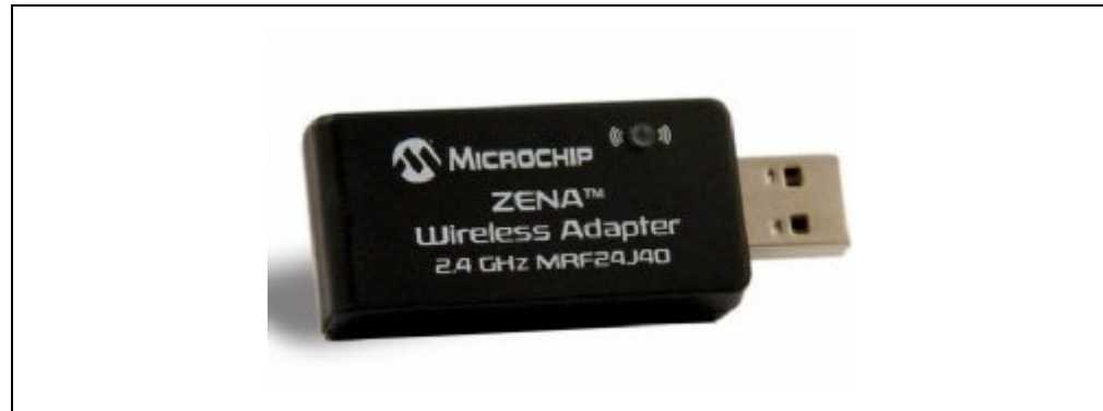
FIGURE 2-2: ZENA™ WIRELESS ADAPTER 2.4 GHZ MRF24J40
