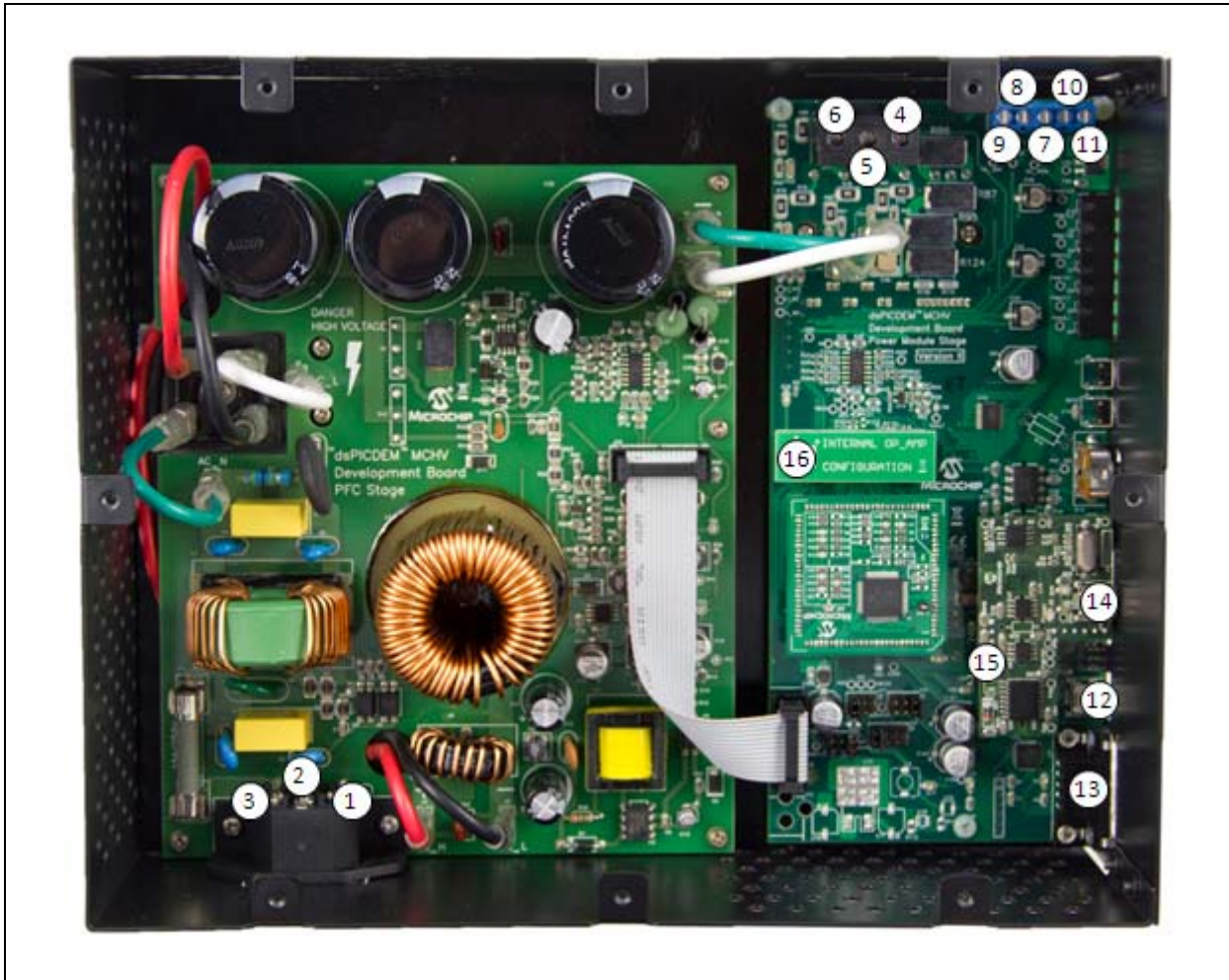
FIGURE 2-5: dsPICDEM™ MCHV-2 DEVELOPMENT BOARD CONNECTIONS
