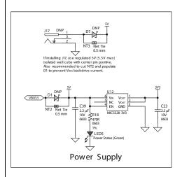
FIGURE A-3: dsPIC33CH CURIOSITY BOARD LAYOUT SCHEMATIC REV. 1.0 (SHEET THREE OF FOUR)
