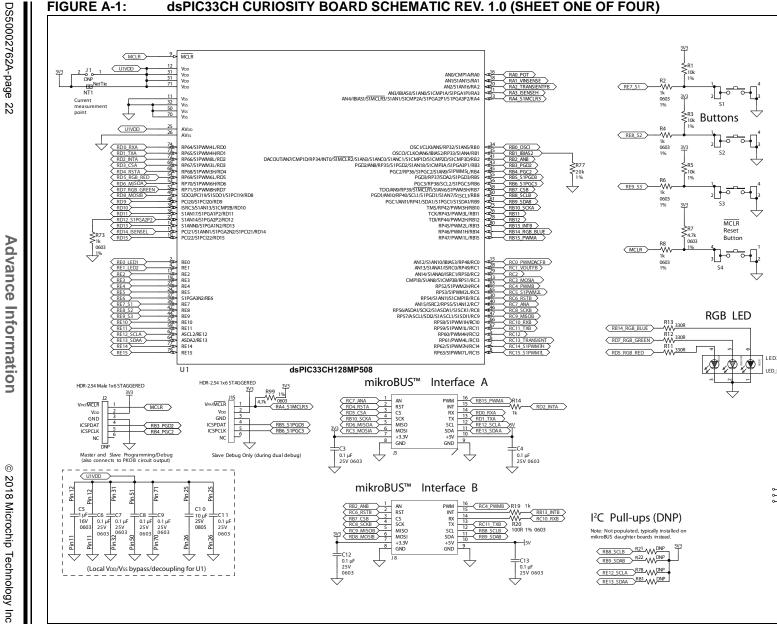
dsPIC33CH CURIOSITY BOARD SCHEMATIC REV. 1.0 (SHEET ONE OF FOUR)
