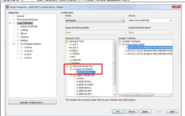
FIGURE 2-1: dsPIC33CH CURIOSITY PKOB TOOL SELECTION
