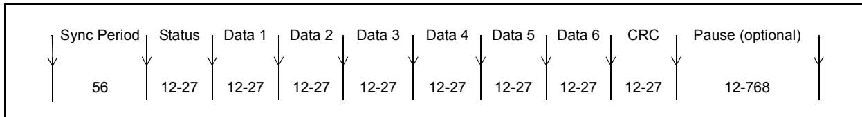
FIGURE 18-2: SENTx PROTOCOL DATA FRAMES
