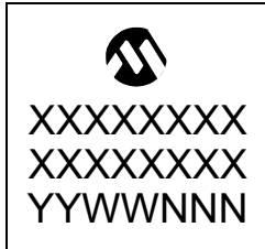
28-Lead UQFN (6x6x0.5 mm)
