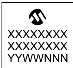
28-Lead QFN-S (6x6x0.9 mm)
