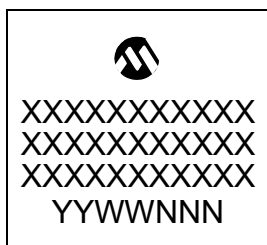
48-Lead UQFN (6x6x0.5 mm)
