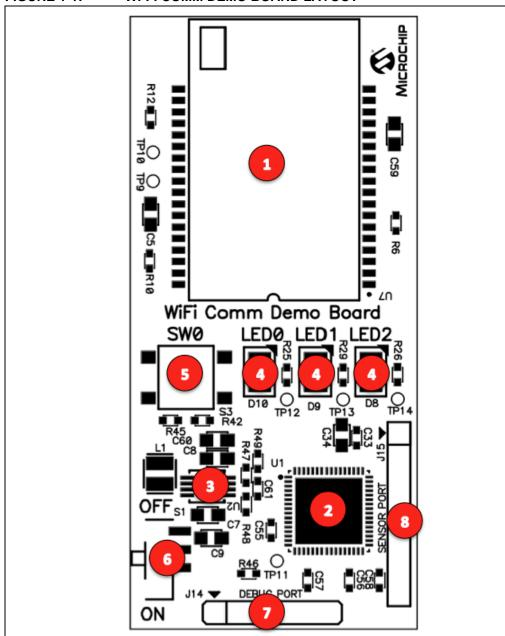
FIGURE 1-1: Wi-Fi COMM DEMO BOARD LAYOUT
